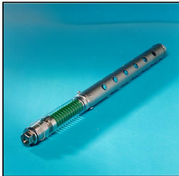
Figure 19: Self stressed tube for combined environment/stress testing
