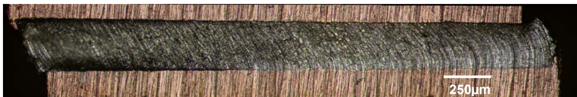
Figure 14. Microstructure of SnAgCu after a creep test (15 MPa at room temperature) coarse grinding marks show localised strain
