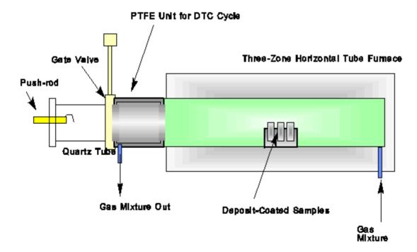
Figure 1 Diagram of the NPL CGA + DTC Testing System
