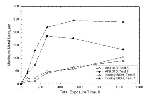
Figure 2 Metal loss as a function of time and test type
