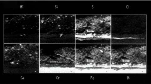
Figure 3 Backscattered electron micrographs and digimap of Incoloy 800H sample with char and salt coating, exposed to CGA+NPL DTC cycles for total exposure time of 70 h
