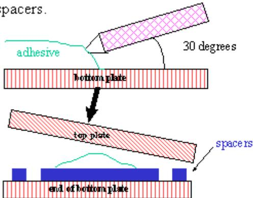
b) When sufficient adhesive has been dispensed, the nozzle is removed and the top plate is then applied.
