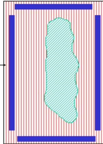
c) The top plate is lowered from one side spreading the adhesive. Pressure is then applied to maintain a uniform thickness during cure.
