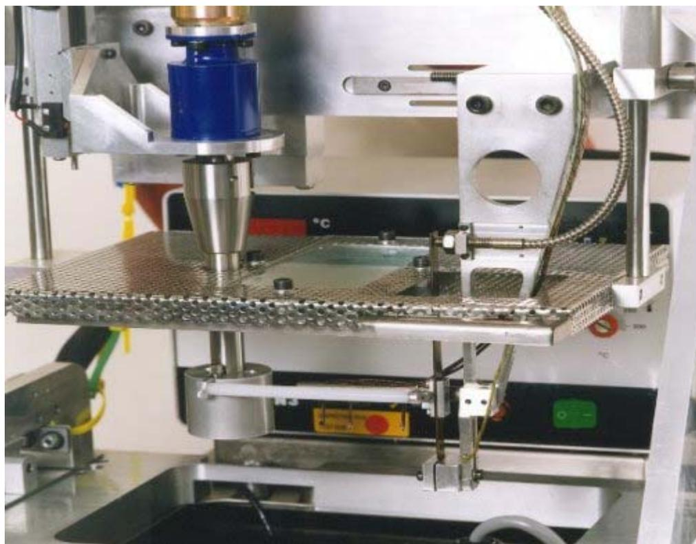
NPL extensile rheometer for measuring the flow properties of polymer melts.
