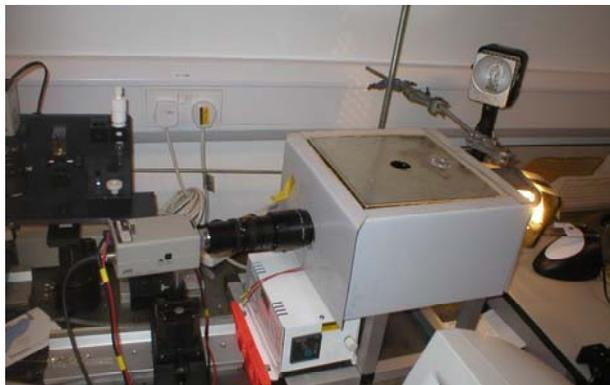
**Figure 9: Apparatus for measuring contact angles of molten hot melts**
