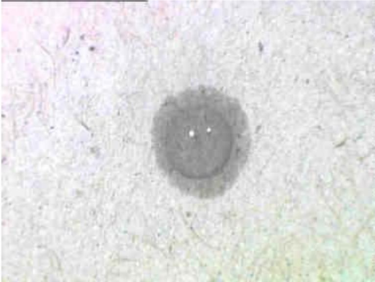
**Figure 22: Liquid drop spreading on a rough, porous surface**
