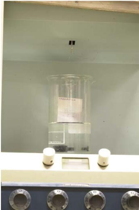
Total immersion tests were considered but it was felt that many of the samples may disintegrate during immersion. Therefore, uptake was determined through an edge absorption/desorption technique.
