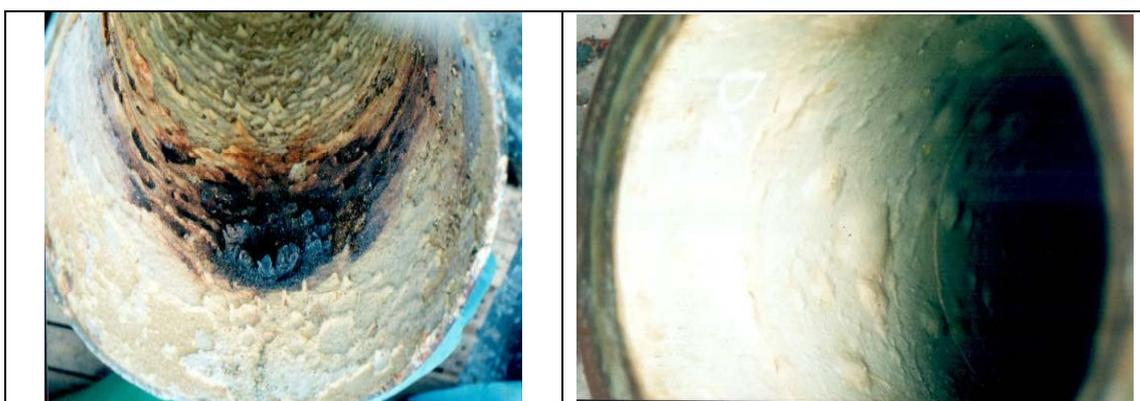
**Figure 3.6:** Chlorine degradation (left) and hydrogen chloride induced blistering (right) of a GRP pipe (courtesy of AEA Technology)
