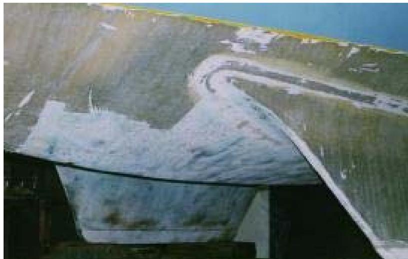
**Figure 3.3:** *Osmotic blistering of a boat hull*
