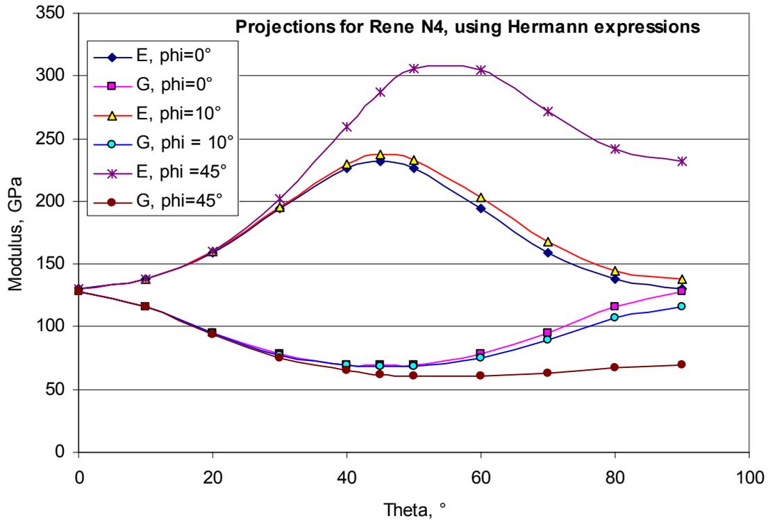
**Figure 2:** Variation in Young's modulus and shear modulus with azimuthal and equatorial angle of direction relative to the crystallographic axes for alloy RENE N4 using compliance data from reference [3] and Hermann's formulation [1].
