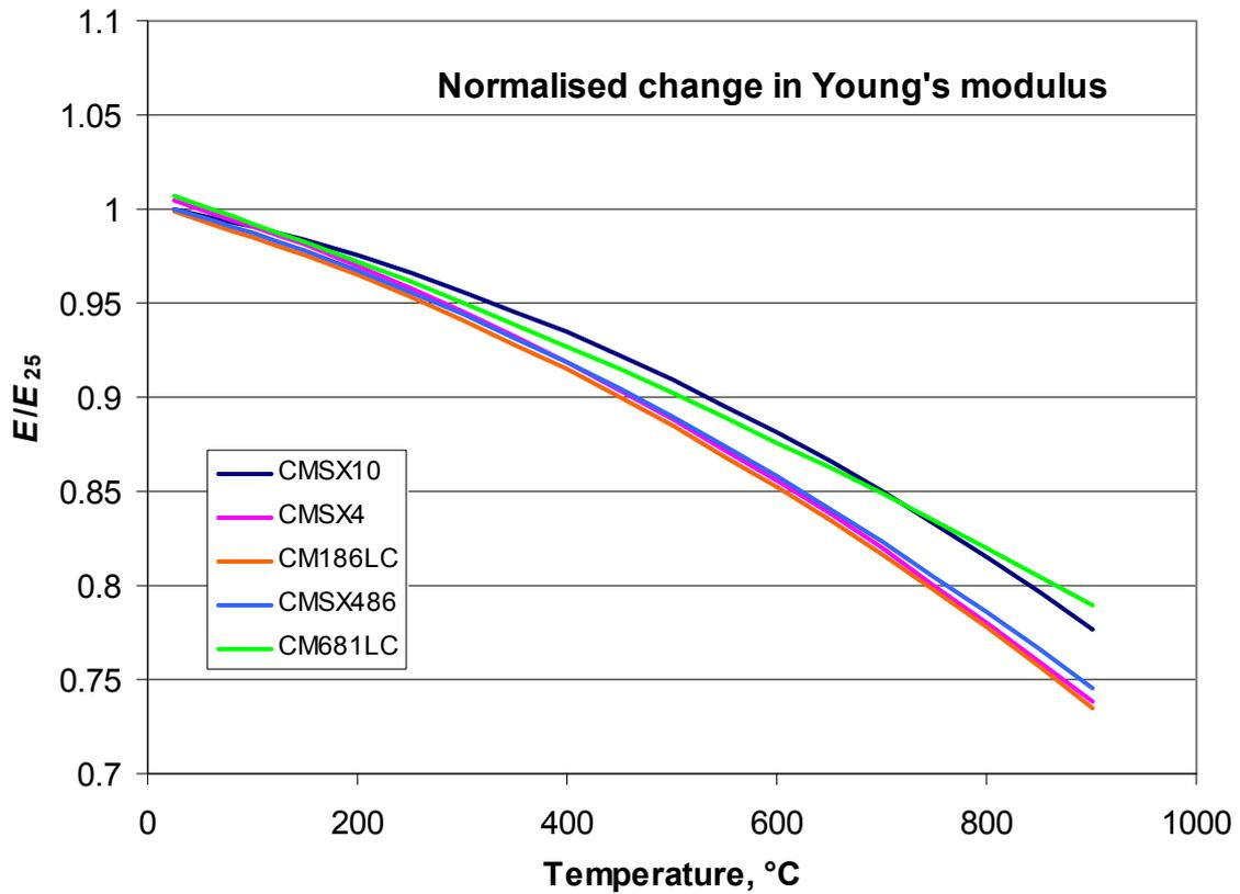
**Figure 3:** Fractional change in Young's modulus close to the [001] direction as a function of temperature for several nickel-based alloys. Also included is the alloy CM681LC cast equiaxially.
