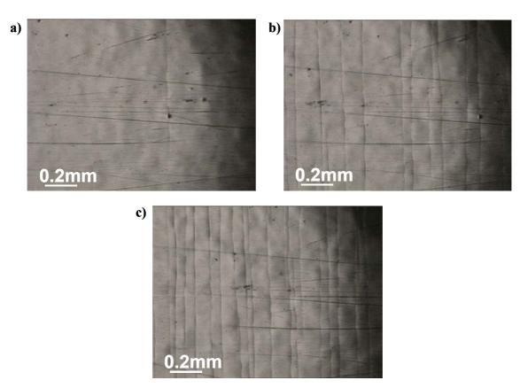
**Figure 8.** Fracture micrographs from tensile test for CrN coated steel with no interlayer. a) 0.65% strain; b) 0.84% strain; c) 1.10% strain. Loading axis was horizontal relative to micrograph. Delamination between substrate and coating is observed before cracking.
