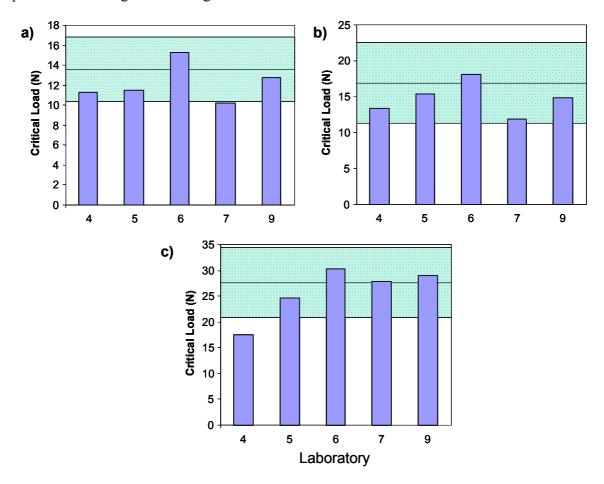
**Figure 7**. ILE critical loads for the BCR-692 diamond-like carbon coated scratch test reference material. Shaded regions indicate upper and lower verification ranges for critical load. a) LC1; b) LC2; c) LC3.
