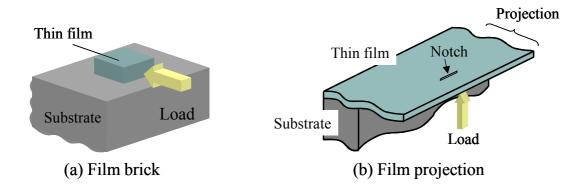
Figure A1. Two specimen configurations
