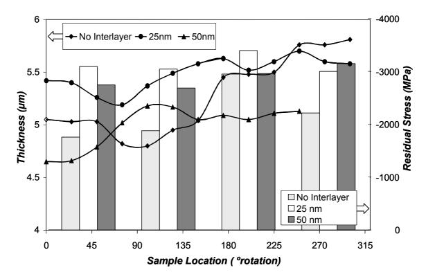
**Figure 4.** Average thickness and residual stress for ILE coupons. Thickness (line chart) was measured on every tenth coupon per batch, position shown relative to 0° line on cassette in Figure 2. Residual stress was measured by XRD on four coupons per batch equispaced around the cassette.
