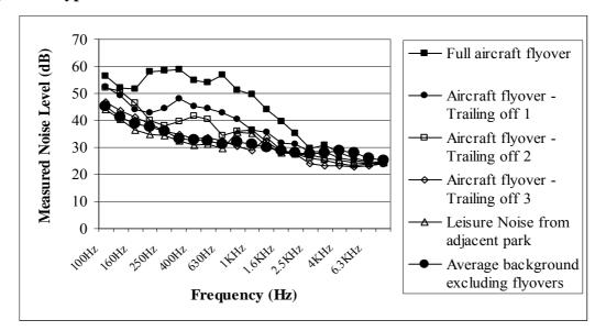
Figure 2. Typical Noise Levels at NPL Test Site
