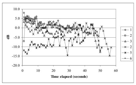
Figure B.6b Sound Power Levels determined over 1-second periods for Shredder/chipper (Long timber samples)
