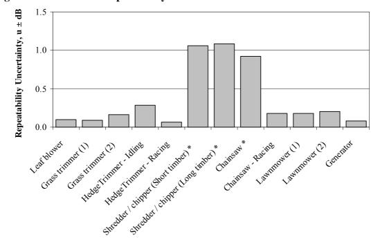
Figure 3. Difference in repeatability between machines
