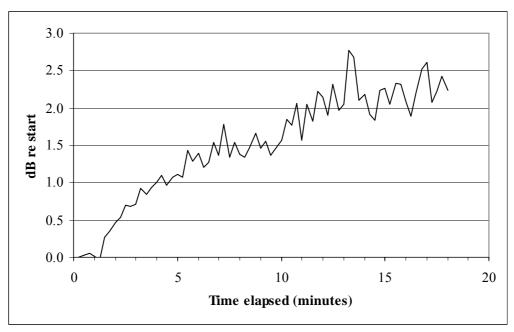
Figure B.5b Sound Power Levels determined over 15-second periods for Hedge trimmer - Racing
