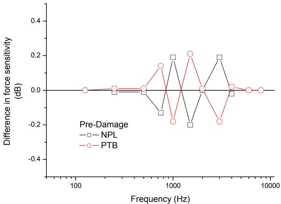
**Figure 5. Difference between mechanical impedance of the mechanical coupler (B&K Type 4930, Serial No. 1895330) measured by participating laboratories relative to the mean difference post-damage.**
