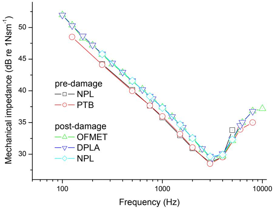
**Figure 2. Results of all participating laboratories showing mean force sensitivity in dB re  $1\text{VN}^{-1}$  of the mechanical coupler (B&K Type 4930, Serial No. 1895330).**
