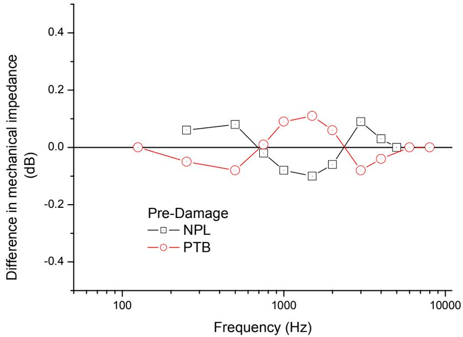
**Figure 4. Difference between force sensitivity of the mechanical coupler (B&K Type 4930, Serial No. 1895330) measured by NPL and PTB relative to the mean difference pre-damage.**
