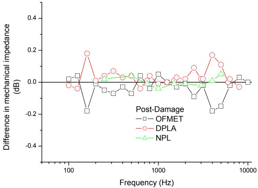
**Figure 6. Difference between force sensitivity of the mechanical coupler (B&K Type 4930, Serial No. 1895330) measured by participating laboratories relative to the mean difference post-damage.**
