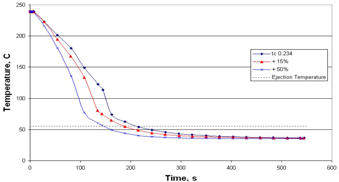
Figure 3 - The effect of different polymer thermal conductivity values on cooling at location T1717 on the pipe ‘T’ piece model.
