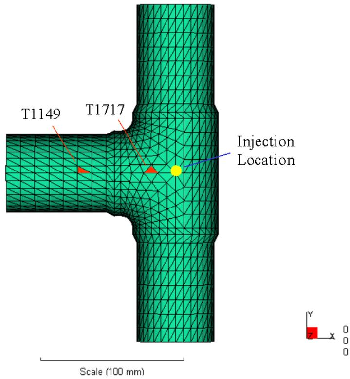
Figure 1 - Pipe 'T' piece model, showing the injection location and two of the locations from which results were obtained.
