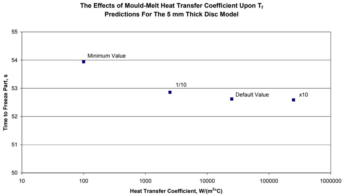
Figure 9 - The effect of different mould-melt heat transfer coefficients upon  $T_f$  for 5 mm thick disc model.
