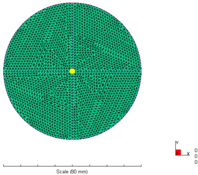
Figure 2 - 80 mm diameter disc model with a central injection location.
