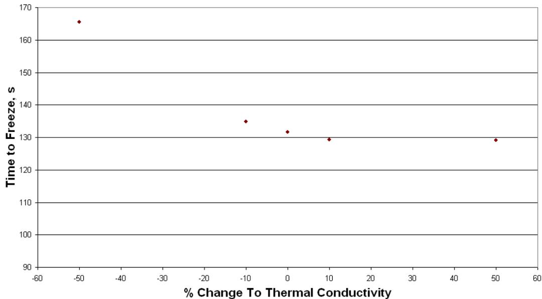
Figure 12 - The effect of different mould thermal conductivity values on  $T_f$  for the pipe ‘T’ piece standard thickness model.
