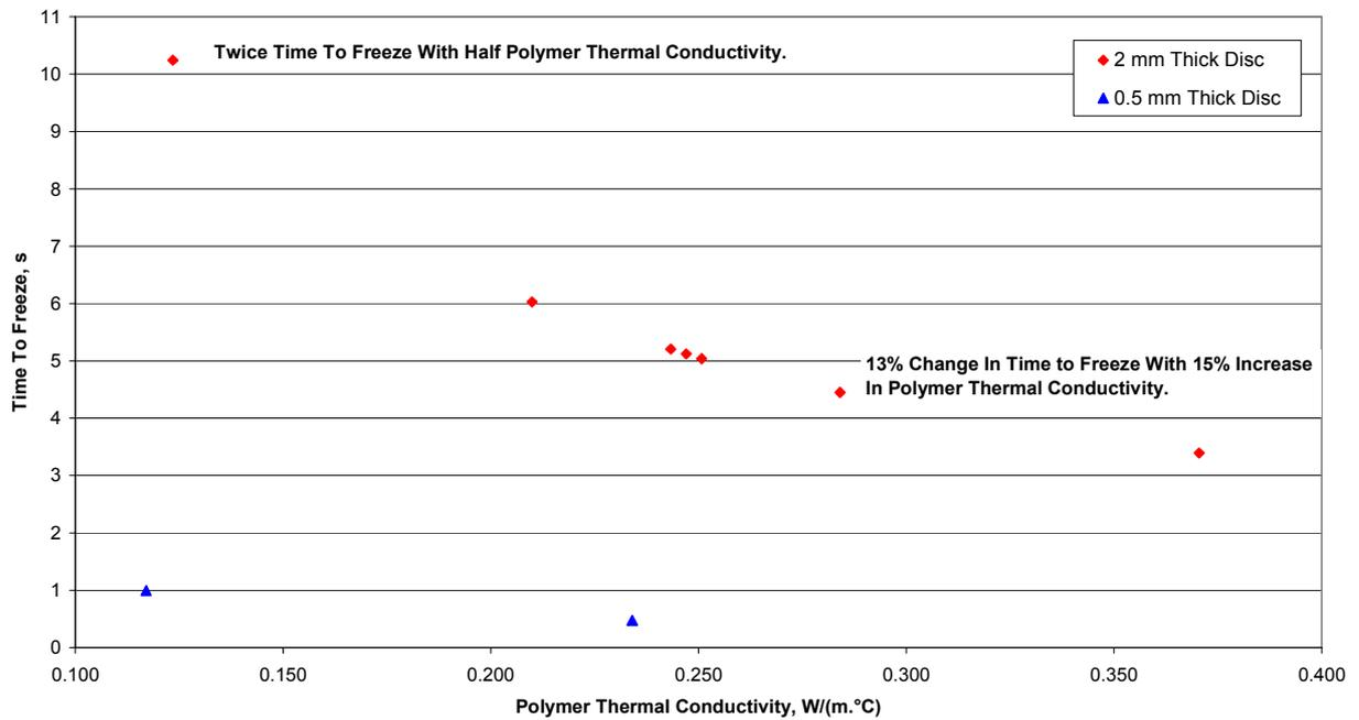
Figure 5 - The effect of different polymer thermal conductivity values upon  $T_f$  for the 2 mm thick disc model with 90°C ejection temperature, and the 0.5 mm thick disc model ejected at 55°C.
