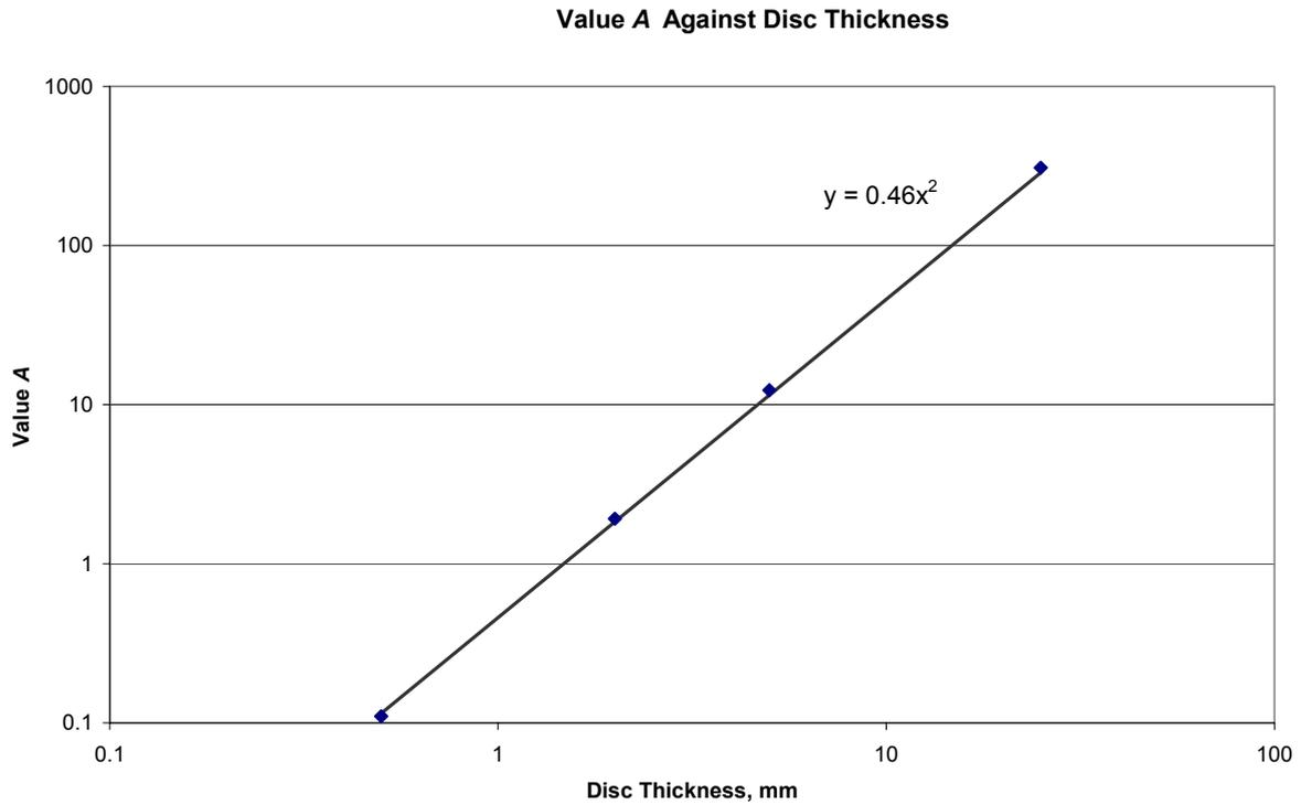
Figure 7 – The relationship between  $A$  and the disc thickness for the simulations with an ejection temperature of  $55^{\circ}\text{C}$ .
