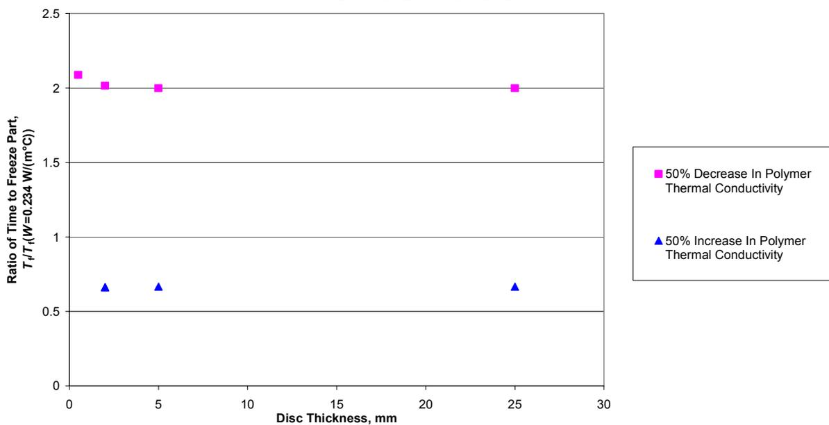
Figure 6 – Normalised  $T_f$  predictions for disc model, thickness from 0.5 to 25 mm and with 55°C ejection temperature, showing the effects of different polymer melt thermal conductivity value. (The predictions for each given disc thickness have been normalised to the prediction from the analysis with polymer thermal conductivity 0.234 W/(m.°C)).
