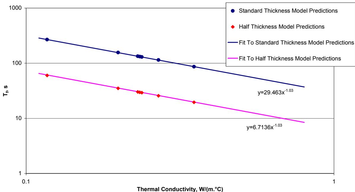
Figure 4 - The effect of different polymer thermal conductivity values on  $T_f$  for the pipe ‘T’ piece model.
