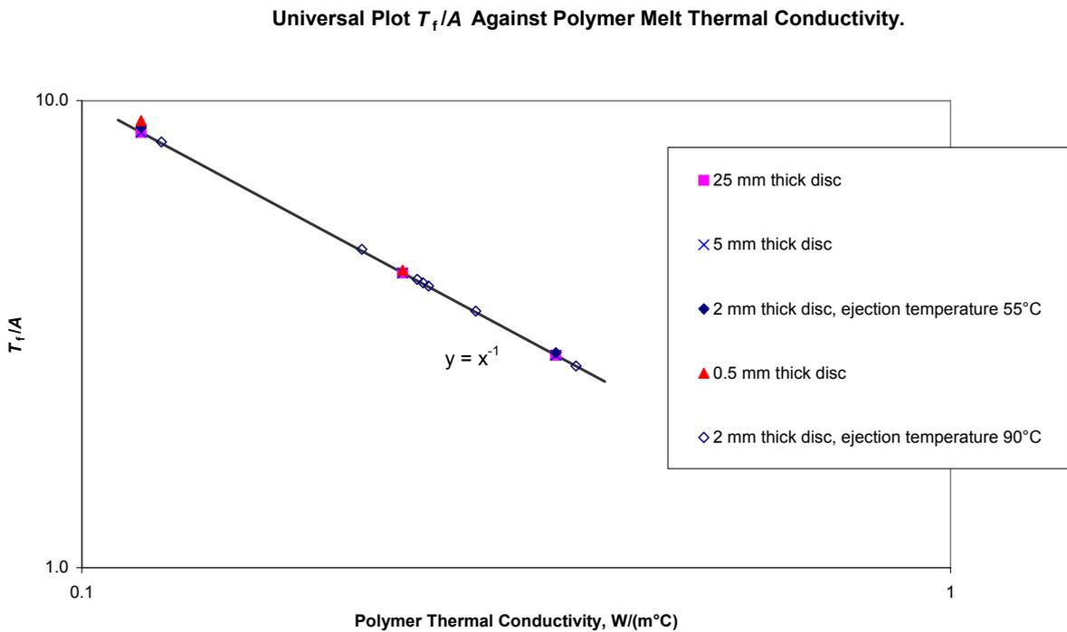
Figure 8 - A universal plot showing the  $T_f$  results from the disc analyses of different thickness normalised using the calculated value  $A$ .
