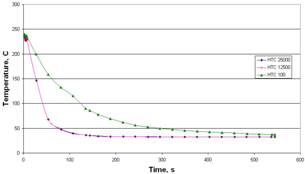
Figure 11 - The effect of different mould-melt heat transfer coefficients upon cooling at location T1149 on the pipe ‘T’ piece model.
