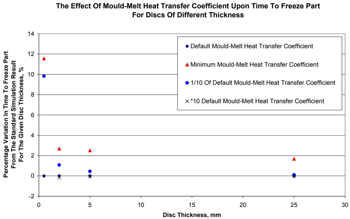
Figure 10 - The relative effect of different mould-melt heat transfer coefficients upon  $T_f$  for discs of different thickness.
