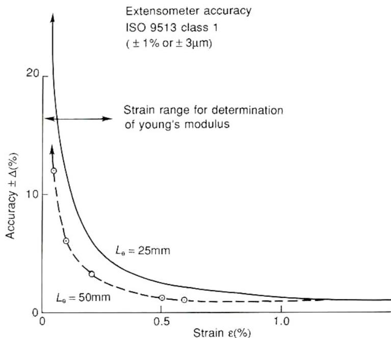
**Fig 2: Typical errors likely in determining Young's Modulus with a Class 1 extensometer [14]**
