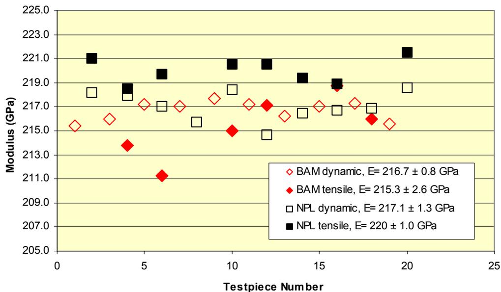
**Fig 1: Modulus data for the BCR Nimonic 75 tensile certified reference material, measured by dynamic and tensile methods.**
