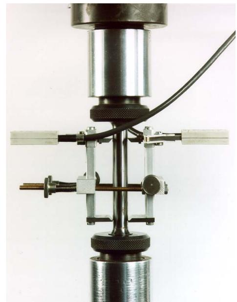
**Fig 3: Typical high resolution averaging extensometer (courtesy of BAM)**
