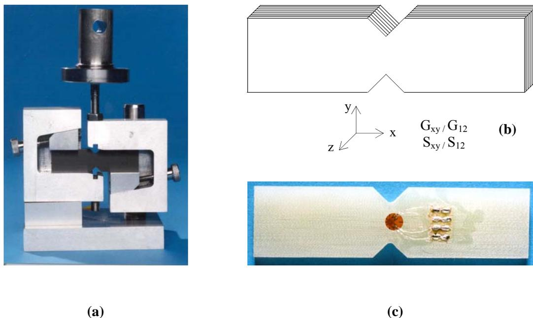
Figure 6 - (a) Iosipescu V-notch beam test rig, (b) fibre axes system for measuring in-plane properties  $G_{xy}/G_{12}$  and  $S_{xy}/S_{12}$ , and (c) specimen with biaxial rosette strain gauge
