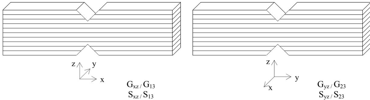
**Figure 9 - Ply orientations of specimens for measurement of through-thickness shear properties**
