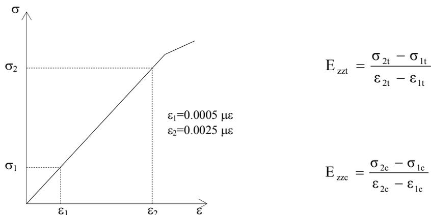
**Figure 8 - Calculation of modulus for through-thickness tension and compression**
