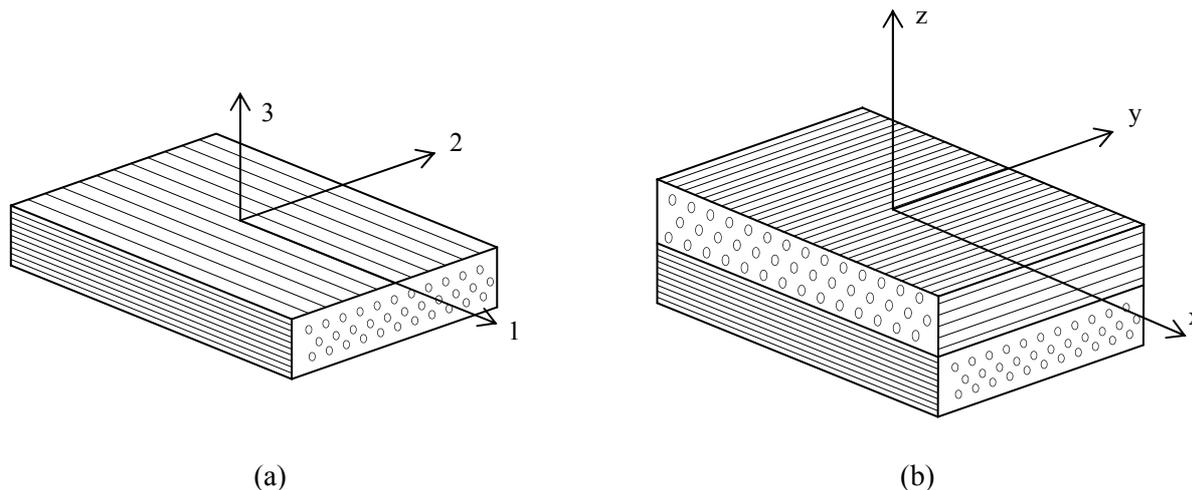
**Figure 1 - Fibre-reinforced plastic composite axes definitions for (a) ply and (b) laminate levels**
