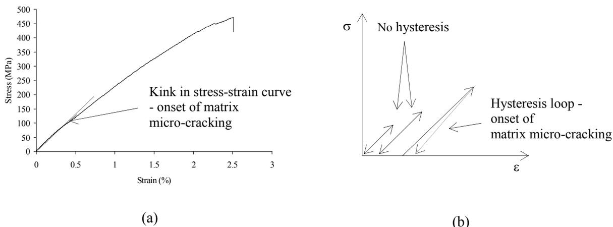
**Figure 4 - Determining the strain limit for onset of matrix micro-cracking**
