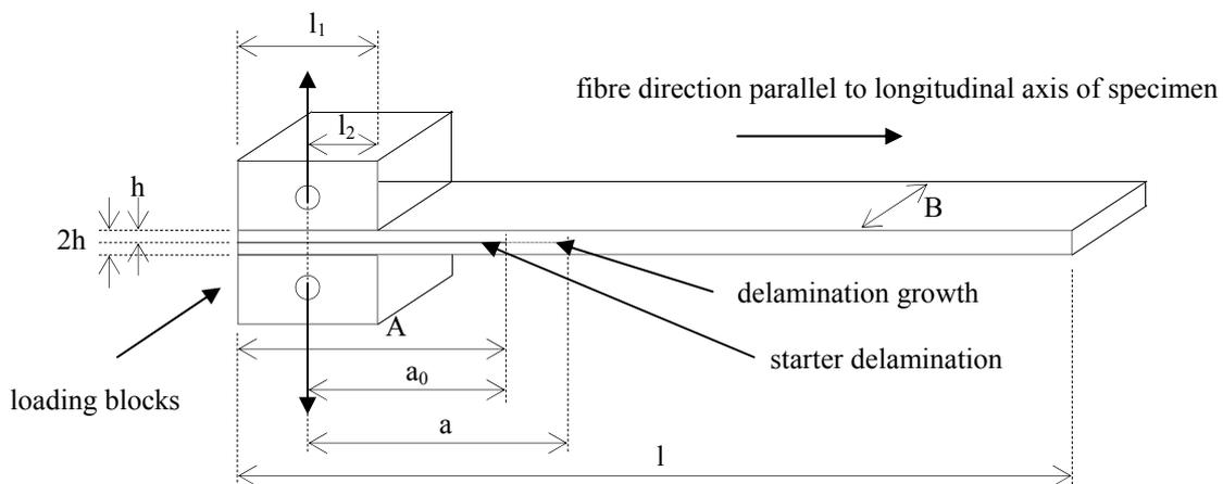
**Figure 10 - Double cantilever beam specimen for measurement of Mode I properties**
