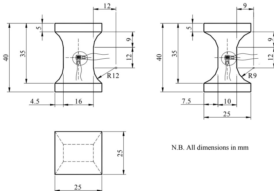
**Figure 7 - RARDE waisted block specimen for through-thickness tension and compression**
