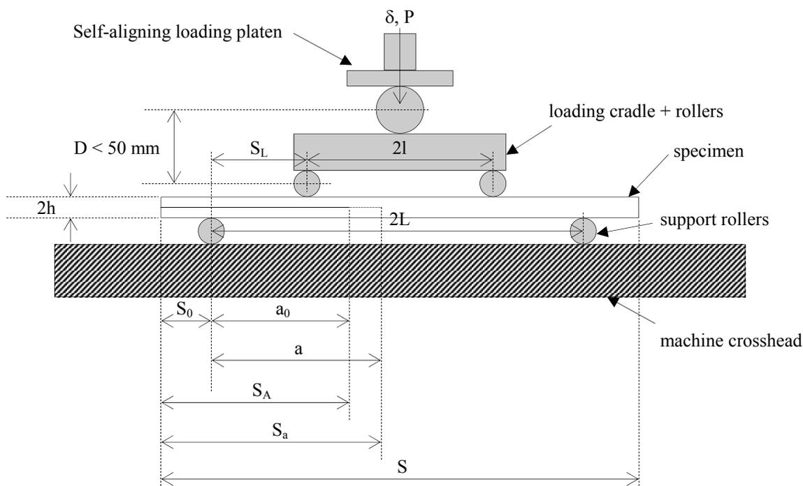
**Figure 11 - 4-point end notch flexure (4ENF) specimen for measurement of Mode II properties**
