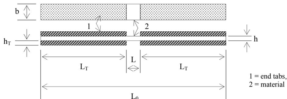
**Figure 5 - Schematic of in-plane compression test specimen for BS EN ISO 14126**
