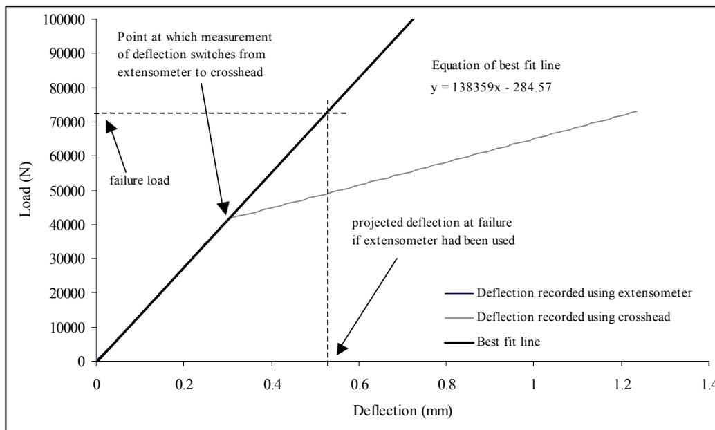
**Figure 3 - Calculation of tensile deflection/strain to failure for plain tensile specimens**
