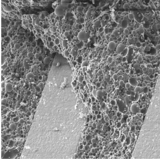
Epoxy based encapsulant (dam and fill) on FR-4 (x55)
