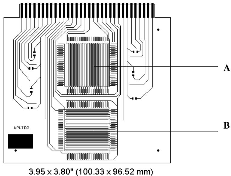
Figure 4: Two dummy QFPs mounted on double comb SIR patterns (A and B) can be used to assess encapsulant adhesion and to monitor moisture permeability during environmental conditioning.
