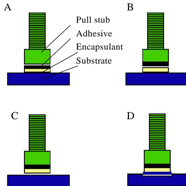
Figure 7: Failure of the encapsulant material can occur at:
