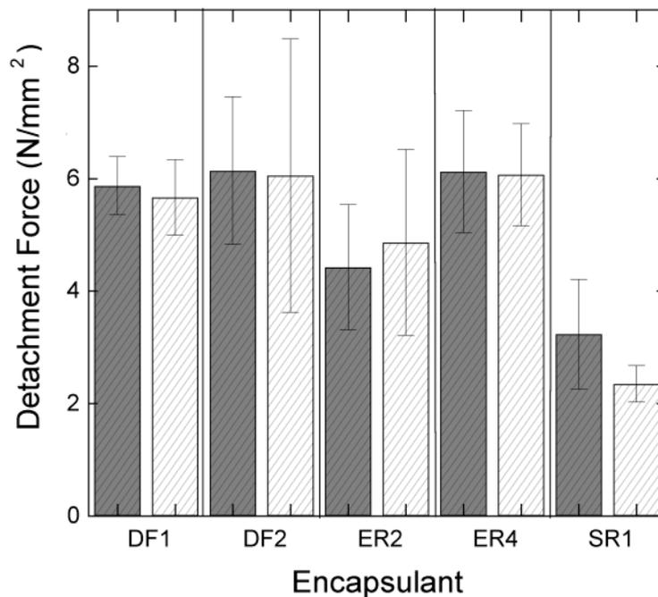
Figure 6: The adhesive strengths of different types of encapsulants (epoxies: DF1, DF2, ER2 and ER4; silicone: SR1) attached to FR-4 can be easily compared in a simple histogram. These data suggest that exposure of the encapsulated board to 100 cycles over the temperature range of  $-40^{\circ}\text{C}$  to  $80^{\circ}\text{C}$  has no influence on thermal strength ( $\square$  = no thermal cycling,  $\blacksquare$  = thermally cycled).
