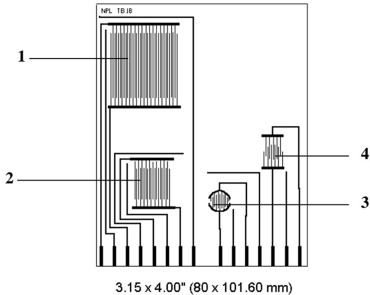
Figure 3: A test board comprising of four double comb SIR patterns labelled 1 to 4.
