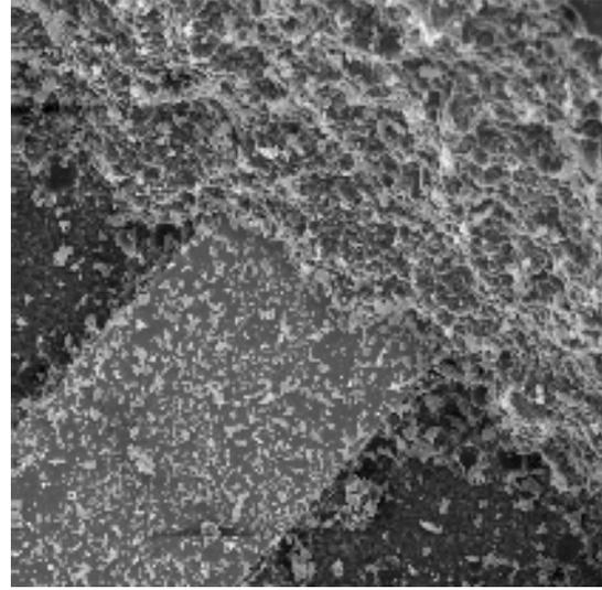
Epoxy based encapsulant on FR-4 (x150)
