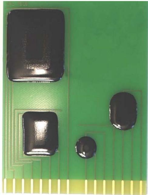
Figure 5: A typical encapsulant (polyurethane) dispensed on to a ceramic board covers not only the double comb areas but also regions of the board coated with solder resist.
