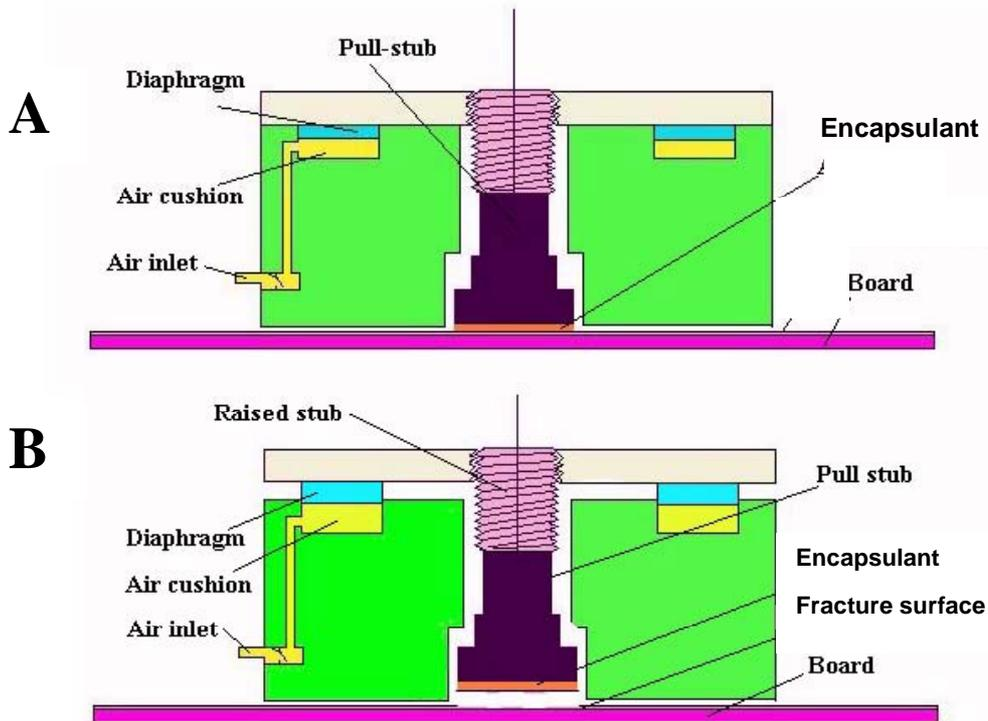
Figure 2: A schematic representation of the butt tension test, A) before and B) after detachment of the pull stub (and encapsulant) from the substrate.
