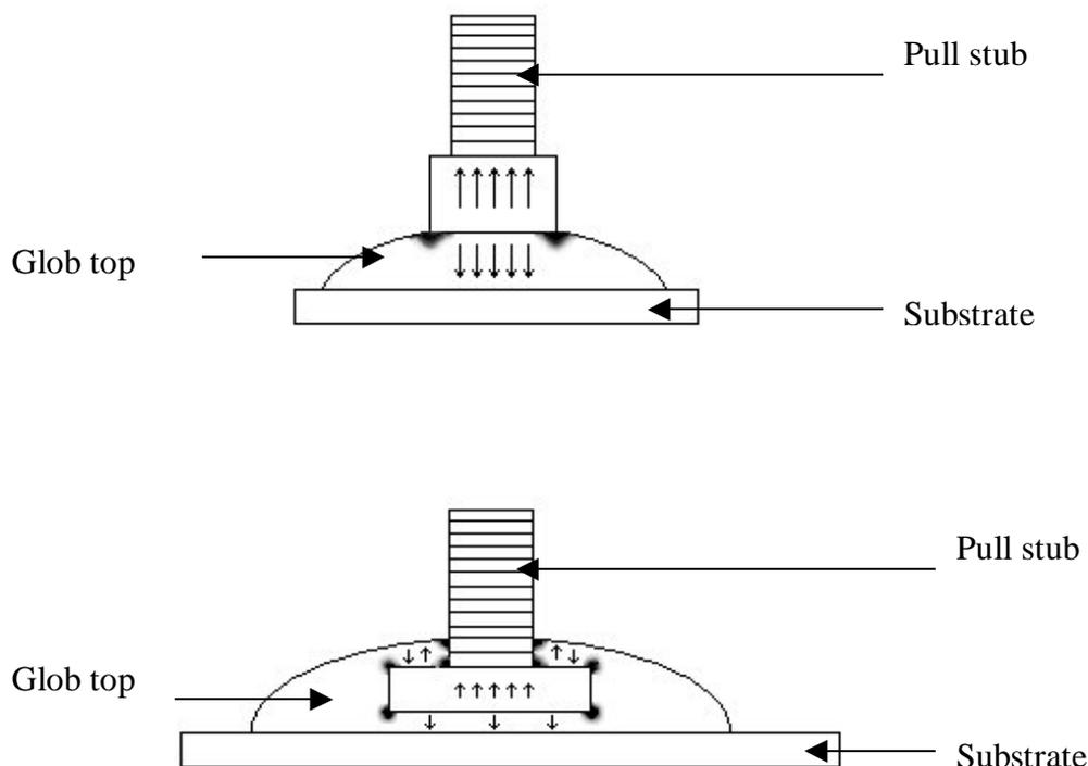
Figure 1: Attaching the pull stub directly to the surface of a cured encapsulant results in some stress concentration around its base (shaded area) and tensile forces within the encapsulant itself (as indicated by the arrows). More stress concentrations occur when the pull stub is embedded in to the encapsulant in addition to compressive stresses.
