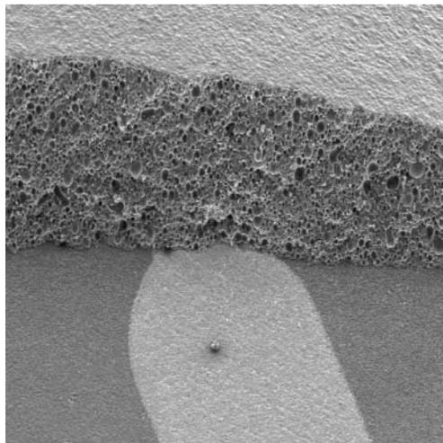
Epoxy based encapsulant on ceramic substrate (x80)
