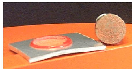
**Figure 2: Pull-Off Specimen**
