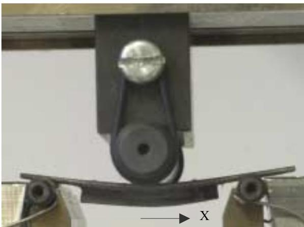
**Figure 10: 3 Point Bend Test**
