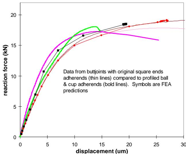
**Figure 5: Butt joint test results**
