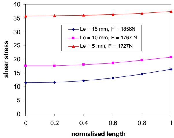
Figure 8: IFSS values calculated for different embedded lengths
