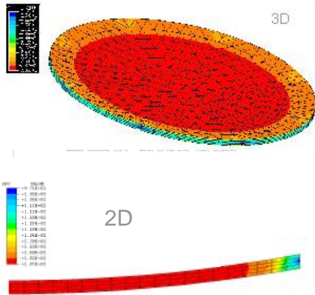
**Figure 4: Stress distribution in modified butt joint**
