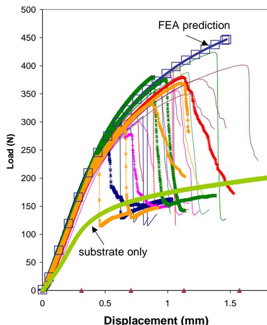
**Figure 11: 3 Point bend results for Adhesive A-aluminium samples**
