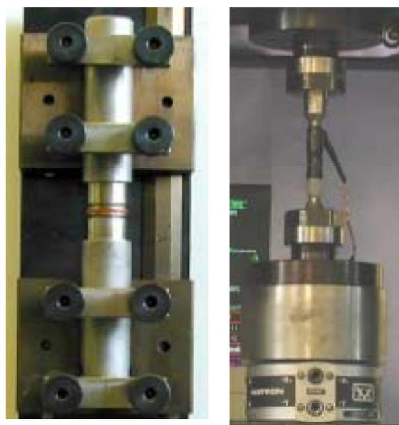
**Figure 3: Butt Joint Sample and Test Alignment**
