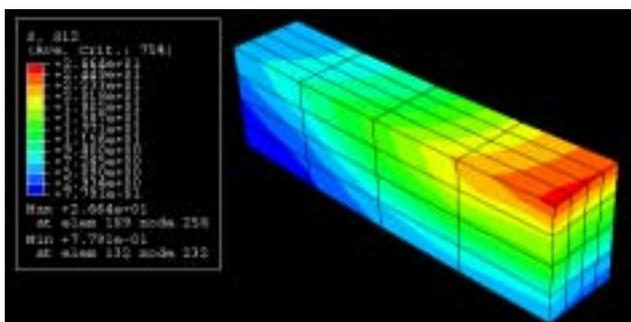
**Figure 12: Shear stress distribution in the adhesive rib. The top of the rib is at the interface between the adhesive and the adherend.**
