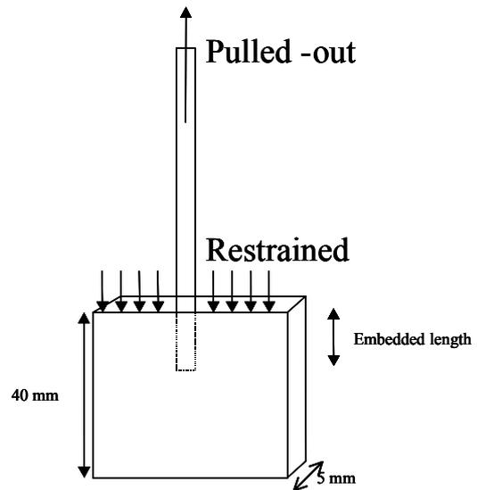
**Figure 6: Pull-out specimen**
