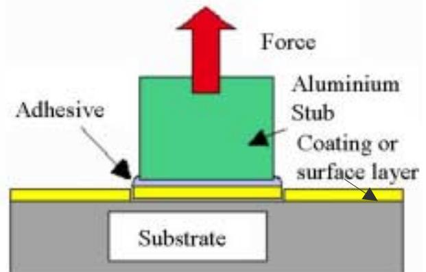
**Figure 1: Pull-Off Test**
