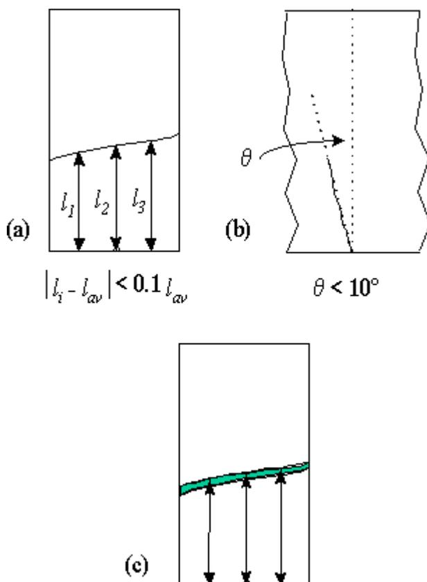
Figure 3 - Acceptable pre-crack geometry, showing criteria for (a) crack length and (b) crack plane angle, and (c) measuring crack length in the presence of subcritical growth.
