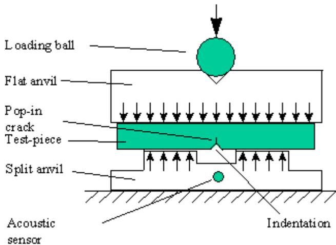
Figure 1 - Schematic of bridge pre-cracking for preparing a single-edge pre-cracked beam test-piece
