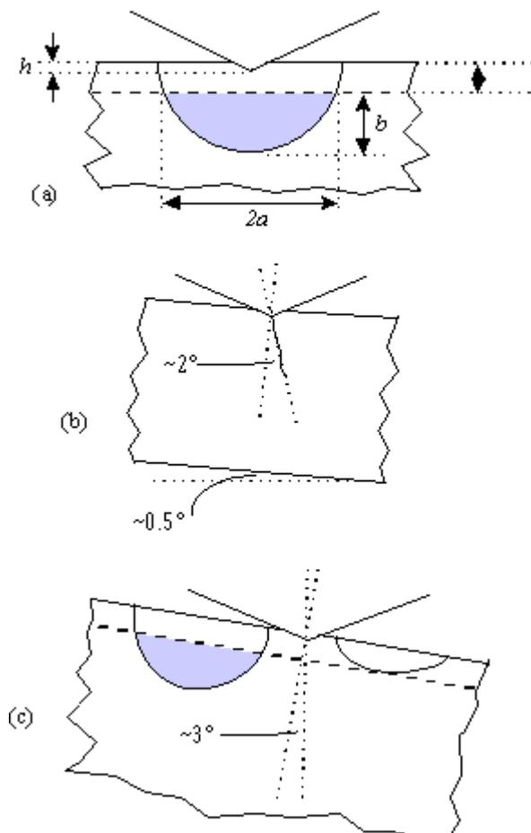
**Figure 5 - Indentation for the surface flaw in flexure method: (a) normal indentation, showing depth of material removal after indentation; (b) enhancement of crack plane angle; and (c) enhancement of Palmqvist crack lobe size in tougher materials**
