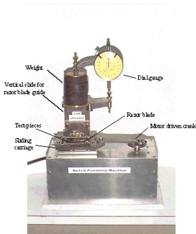
Figure 4 - Reciprocating notch honer based on a sliding table and a guided razor blade
