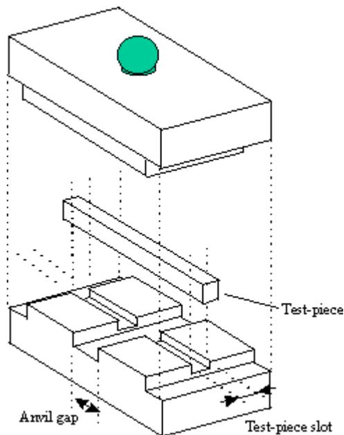
Figure 2 - Example of a pre-cracking jig for the SEPB method
