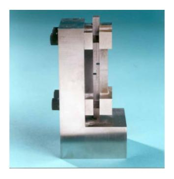
Figure 3 Specimen in anti-buckling fixture
