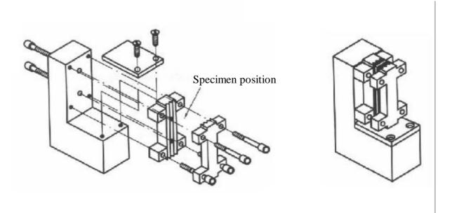
Figure 2 Schematic of anti-buckling fixture
