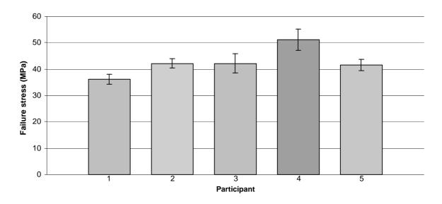
Figure 5 Comparison of average failure stresses (with error bars) of specimens manufactured with Adhesive B from each participant
