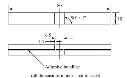
Figure 1 Thick adherend shear test compression specimen dimensions
