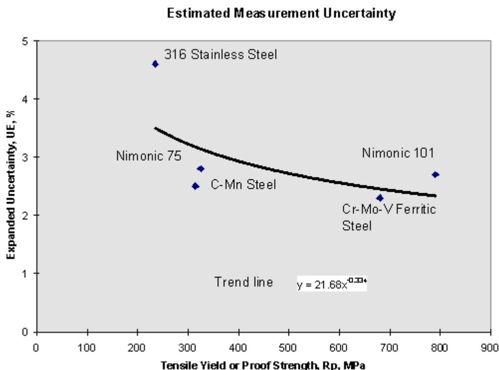
Figure 1. Expanded Measurement Uncertainties at the 95% confidence level for Proof or Yield Strengths selected materials tested in accordance with EN 10002 Part 1
