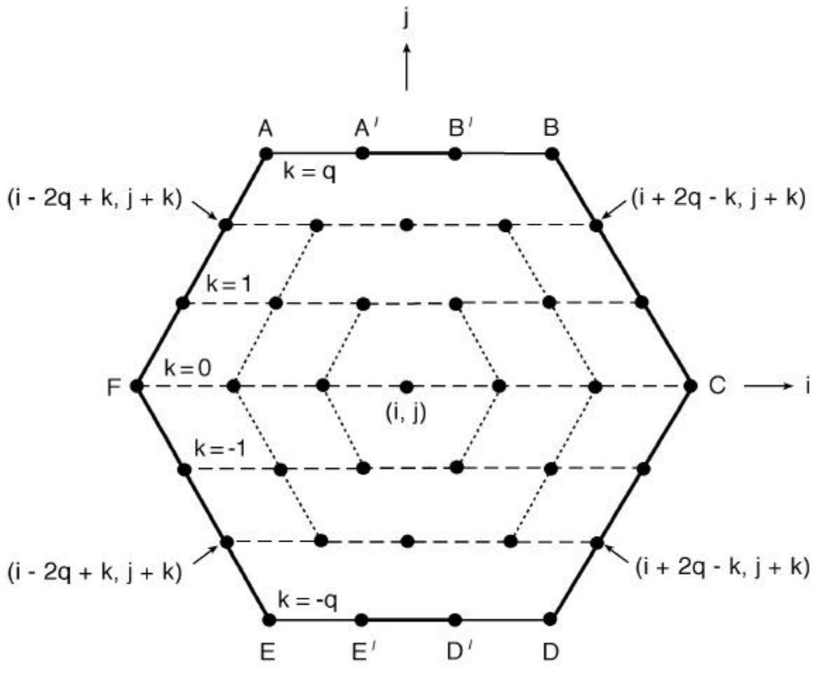
Fig.3 : Diagram defining the hexagonal rings around a fibre element located at  $(i, j)$
