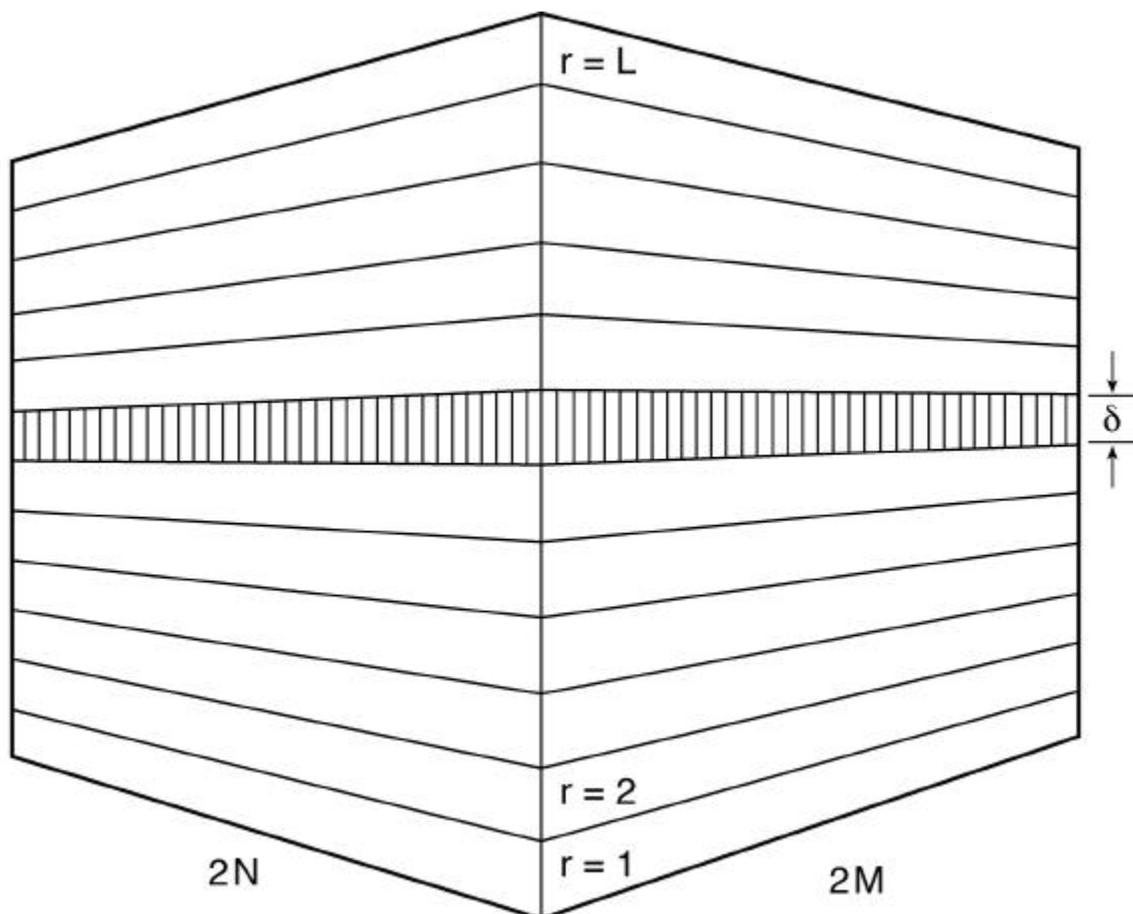
Fig.1 : Schematic diagram of a unidirectional composite that is divided into layers of equal length  $d$
