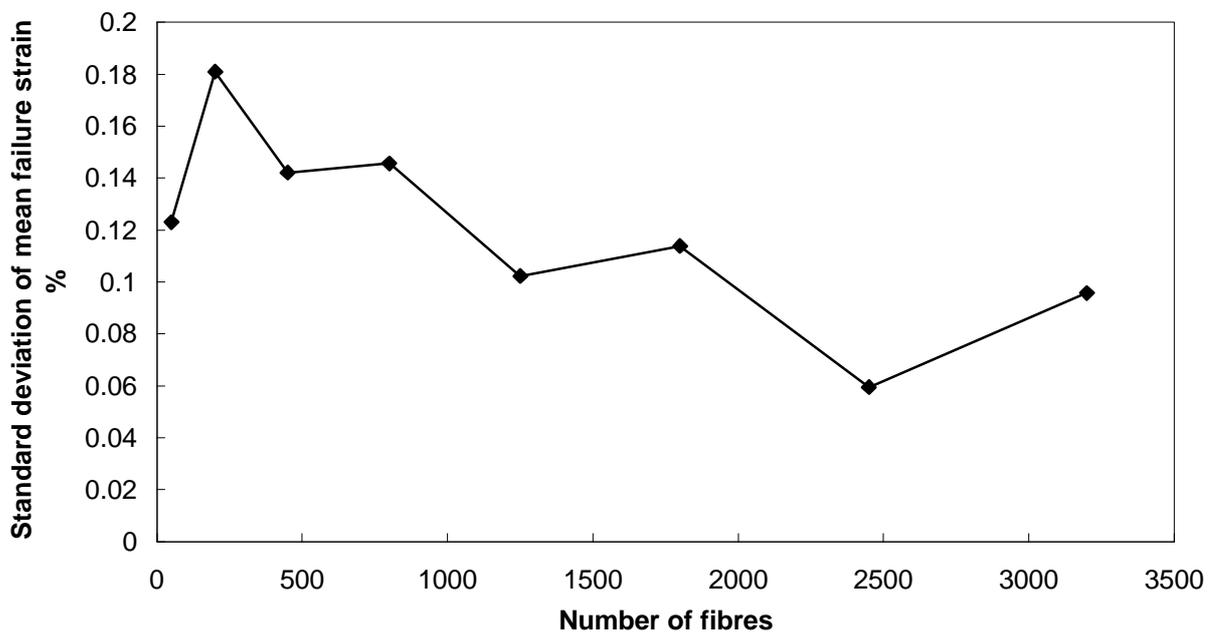
Fig.6 : Dependence of standard deviation of mean failure strain as a function of the number of fibres in the simulation.
