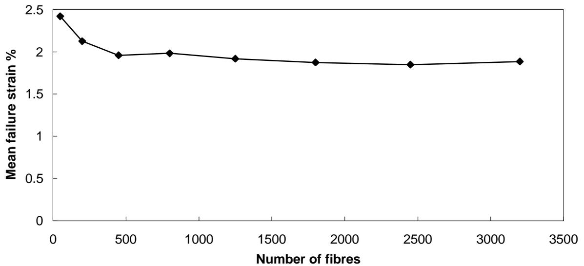
Fig.5 : Dependence of mean failure strain as a function of the number of fibres in the simulation.
