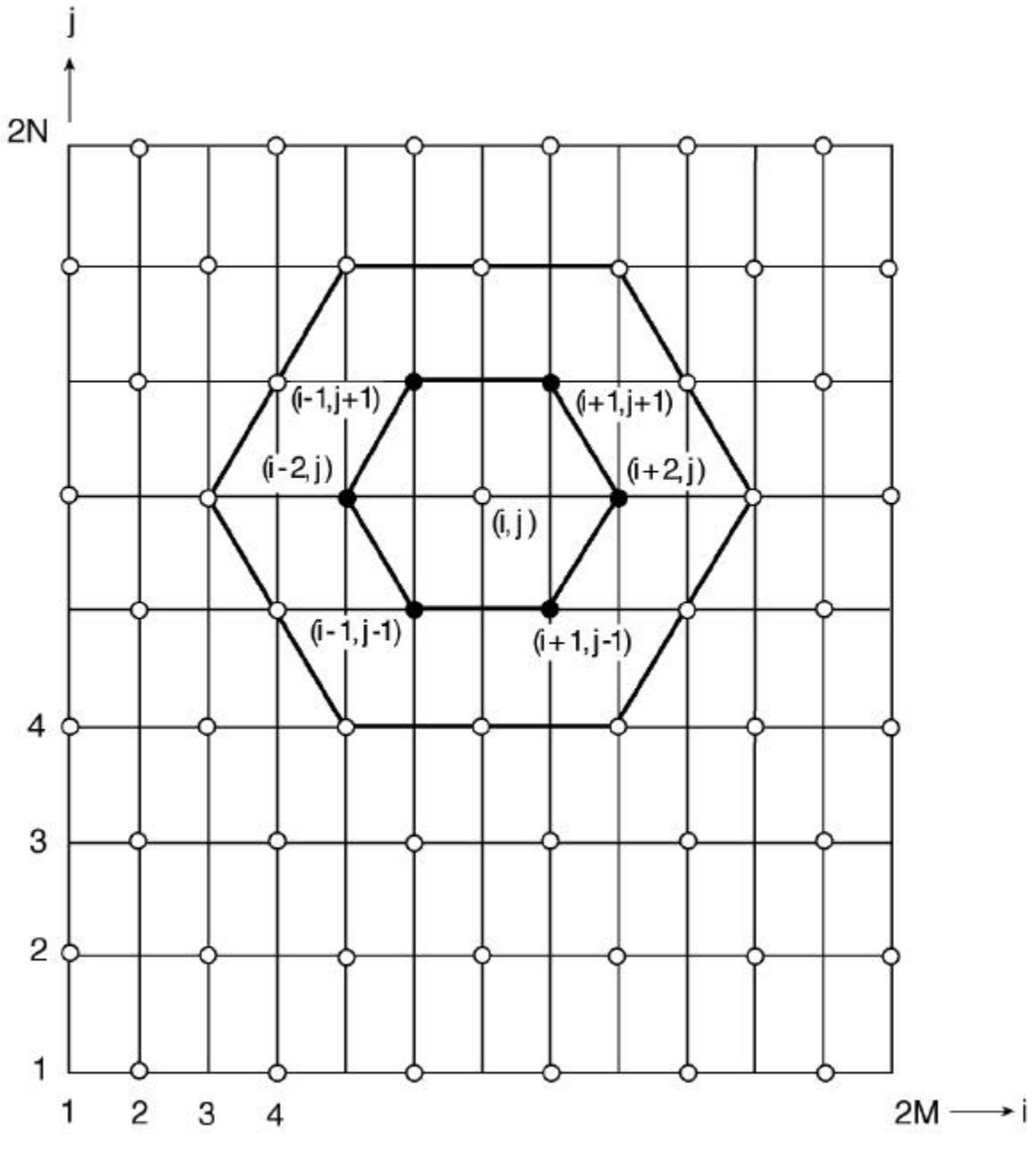
Fig.2 : Rectangular grid on which fibres are located having a hexagonal distribution
