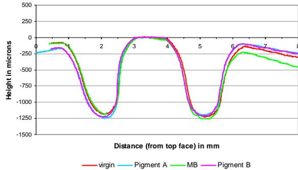
Figure 8 - Raw laser profilometer data for different pigmented feedstocks.
