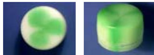
**Figure 2 - Mould filling flow front patterns.**
