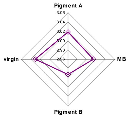
**Figure 10 - ANOM plot of influence of pigment type on cap weight (g).**
