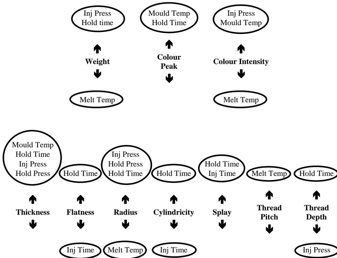
Figure 16 - Control diagram depicting the statistically significant processing variables which affect non-geometric quantities (upper) and geometric quantities (lower).
