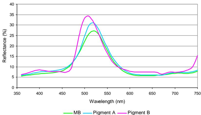
**Figure 12 - Typical raw data colour spectra for different green pigments.**
