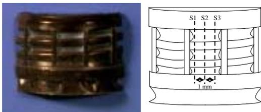
**Figure 5 - Thread measurements, S1 to S3.**
