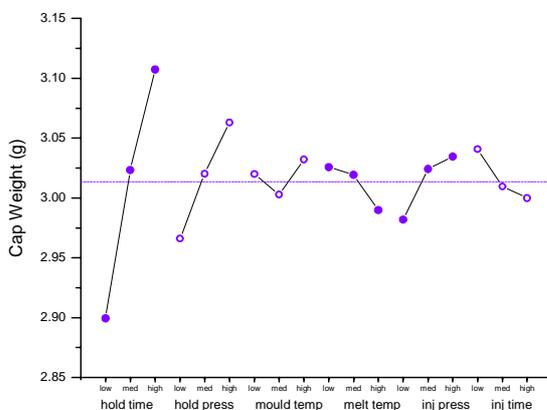
**Figure 9 - ANOM plot of influence of process variables on cap weight.**
