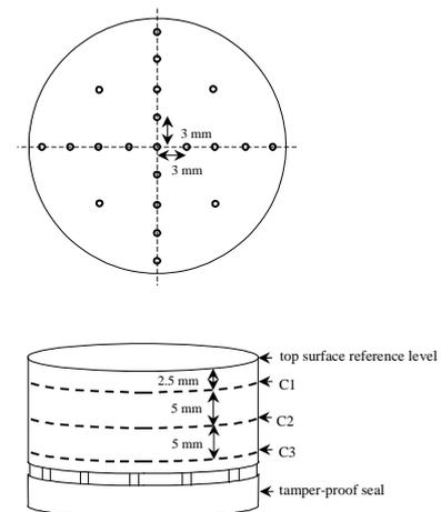
Figure 4 - CMM measurements: (top) flat face and (bottom) perimeter C1 to C3.
