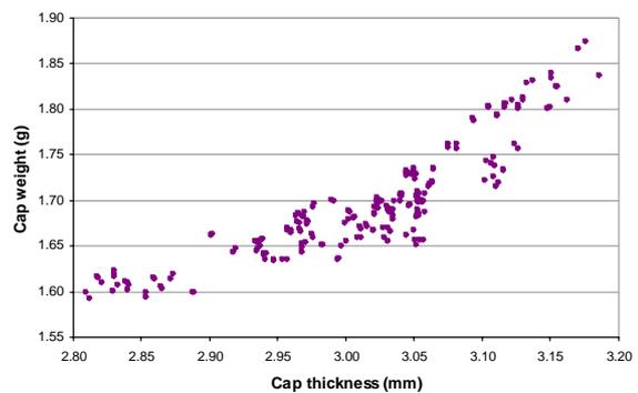
**Figure 11 - Plot of weight against thickness for all individual caps.**
