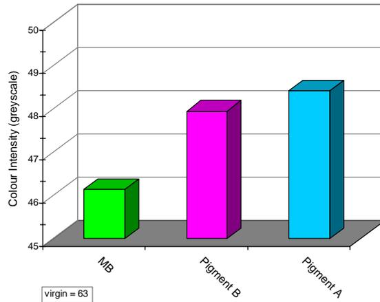
**Figure 13 - ANOM plot of influence of pigment on colour intensity (greyscale).**
