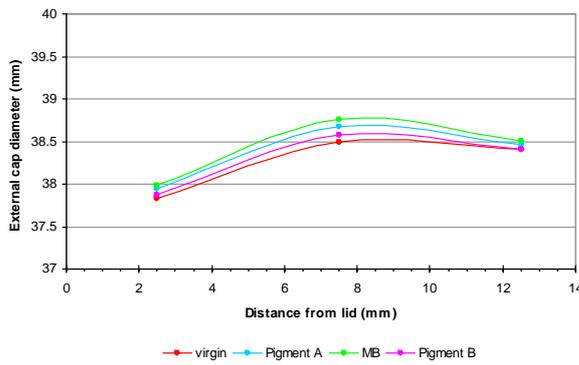
Figure 15 - Curved cap wall profiles for different pigments.
