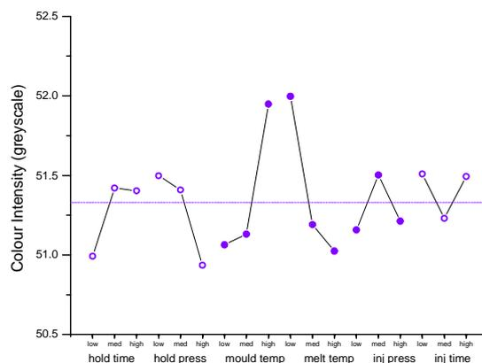
**Figure 14 - ANOM plot of influence of process variables on colour intensity.**
