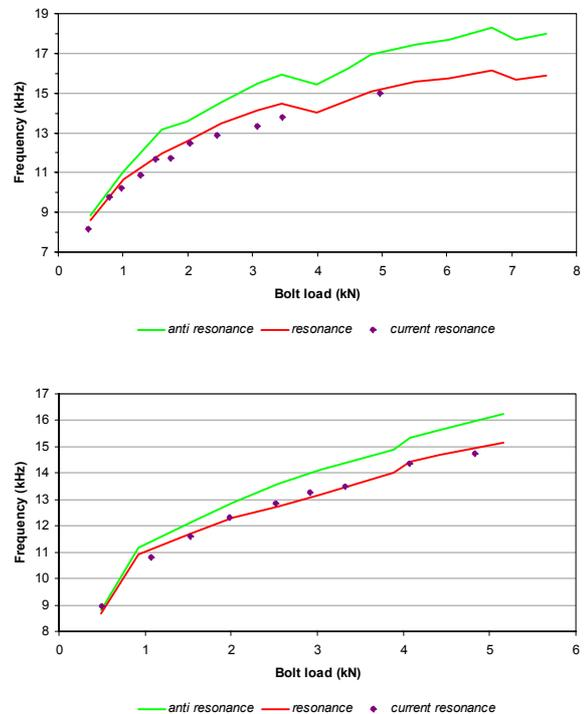
**Figure 11 - Comparisons between resonance and anti-resonance impedance data and current resonance data with increasing clamping load: (a) Channel 5400 and (b) PC8.**
