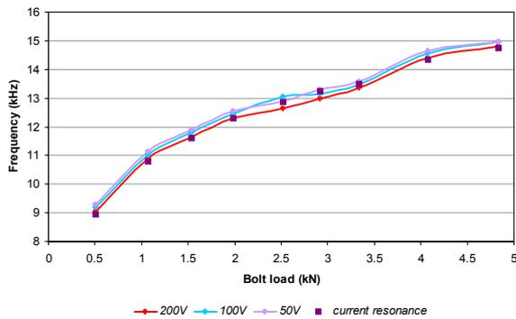
**Figure 13 - Comparisons between resonance from current and displacement data with increasing clamping load for PC8.**
