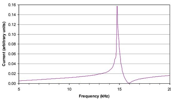
**Figure 9 - Typical current measurement at high field (example from PC8 at 5kN bolt load, 200 V pk-pk).**
