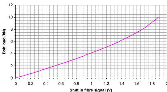
Figure 3 - Typical fibre output calibration trace.
