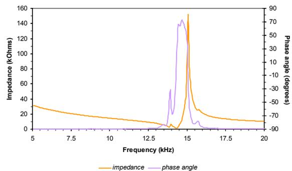
Figure 7 - Typical impedance and phase angle measurements at low field (example from PC4D at 4kN bolt load, 1 V pk-pk).
