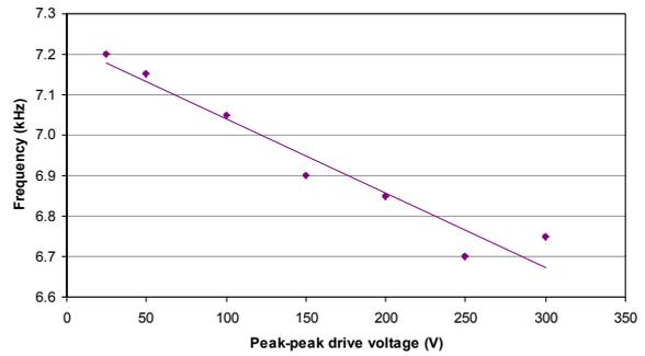
**Figure 10 - Relationship between current resonance frequency and driving voltage amplitude (example from PC8 at <500N bolt load).**
