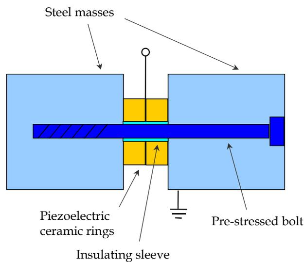
**Figure 1 - Typical sonar sandwich transducer configuration.**
