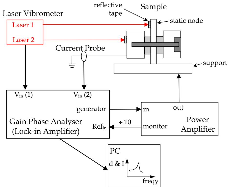
Figure 6 - Schematic of high field displacement and current measurement set-up.
