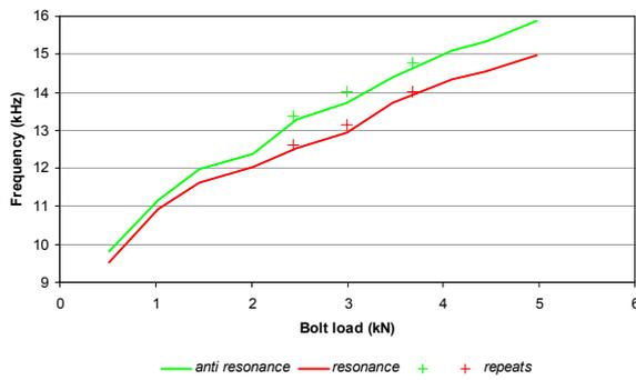
**Figure 8 - Resonant and anti-resonant frequencies for PC4D.**
