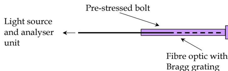
**Figure 2 - Schematic of an instrumented bolt.**
