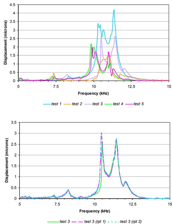
**Figure 16 - Raw vibrometer displacement data for PC8 at 1.5 kN pre-load and 200V: (a) rotating piezo rings between each test and (b) repeats with no changes to set-up.**
