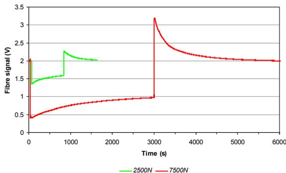
**Figure 5 - Decay in fibre signal due to creep at different load levels.**
