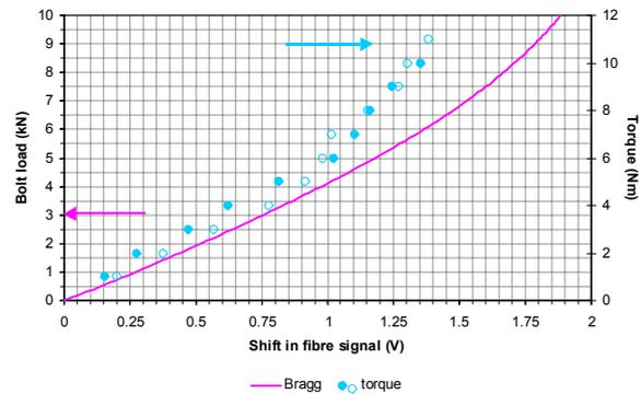
Figure 4 - Comparison between actual bolt load and torque level loading.
