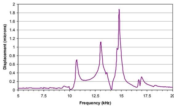
**Figure 12 - Typical vibrometer displacement measurements at high field (example from PC8 at 5kN bolt load, 200 V pk-pk).**
