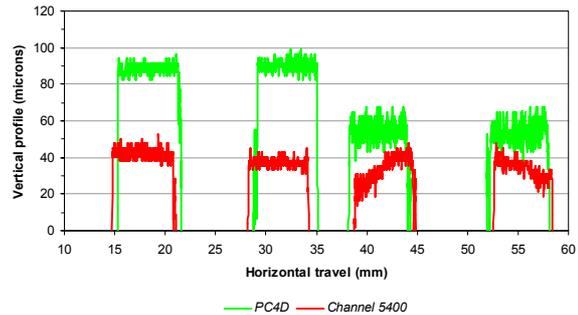
**Figure 15 - Surface profiles of PC4D and Channel 5400 rings.**
