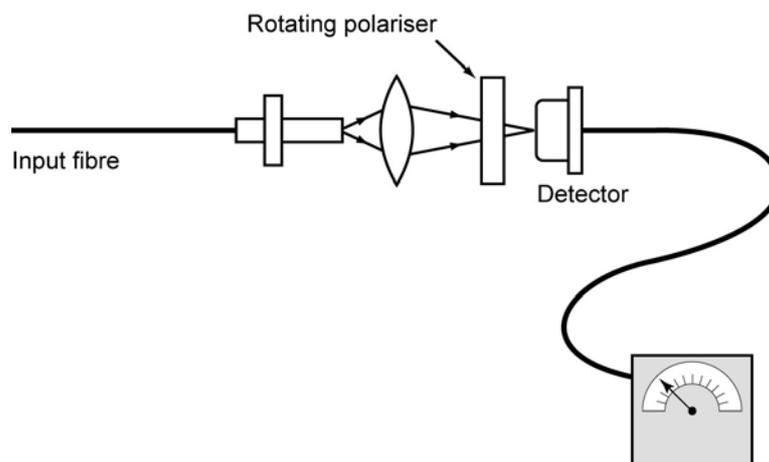
Figure 4. Polarisation extinction ratio meter in diagrammatic form.
