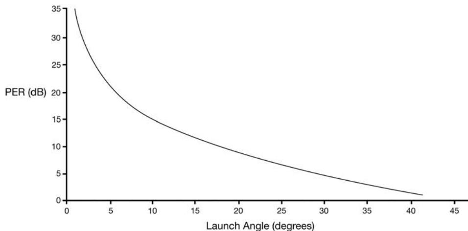
Figure 5. PER values calculated as a function of launch angle offset to the slow axis.
