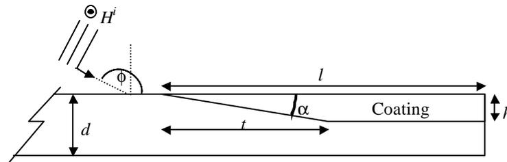
**Figure 1** A coated conducting halfplane edge illuminated by an H-polarized wave. The dielectric coating has a relative permeability of  $\mu_r=1$  and a relative permittivity  $\epsilon_r$ . The coating has a taper of length  $t$  at its front edge, a total length of  $l$  and thickness  $h$ .  $0 \leq t \leq l$ .
