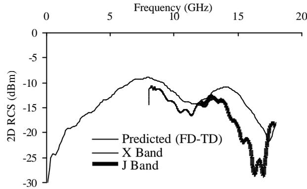
**Figure 2** Measured and predicted data of a coated edge.
