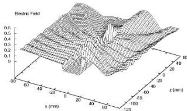
**Figure 3** 3\_D representation of the magnitude of the Efield near the rear end of the test-piece, which is positioned at  $x = 0, z < 0$ . The dielectric taper is positioned in the quadrant  $x > 0, z < 0$ , as are the fields above it. The finite size of the OMS prevents it from measuring in the rectangular region close to the test-piece shown with zero field. The vertical axis shows the electric field in arbitrary units.
