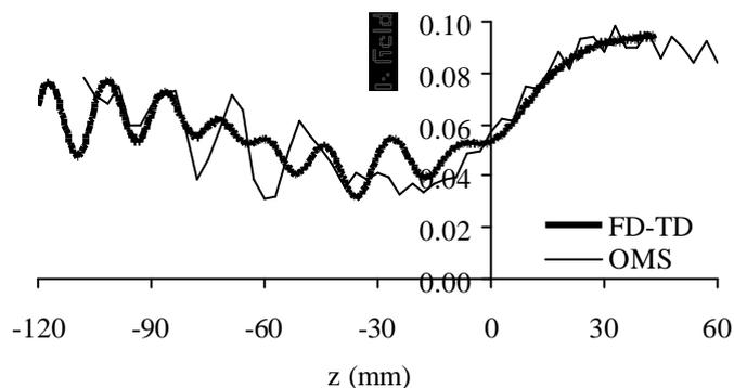
**Figure 4** A comparison between the measured (OMS) and predicted E field magnitude 19 mm above the lossless coating. The vertical axis shows the electric field in arbitrary units.
