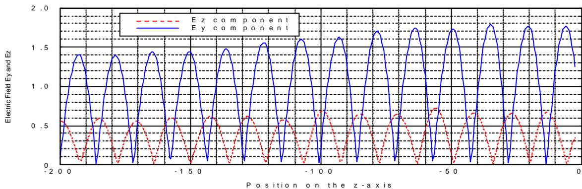
**Figure 3** Comparison between  $E_y$  and  $E_z$  for a  $z$ -scan.  $z = 0$  corresponds to the position of the conducting waveguide termination, see Figure 1. The vertical scale is in arbitrary units but  $E_y$  and  $E_z$  are correctly scaled with respect to each other.
