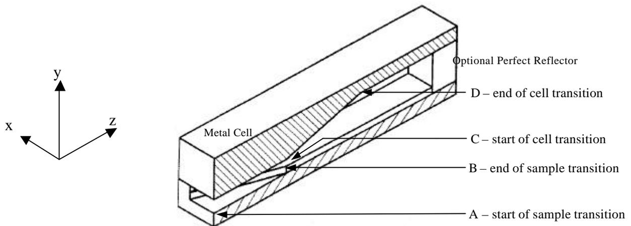
**Figure 1** Schematic diagram of a section through the electromagnetic surface wave cell
