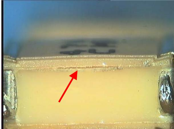
**Figure 17. Cracks in the end of the Polyester Capacitor.**
