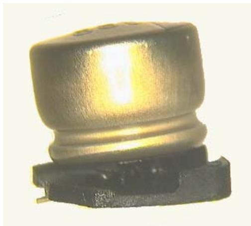
**Figure 18. 100 $\mu$ F Electrolytic Capacitor after LF Reflow**
