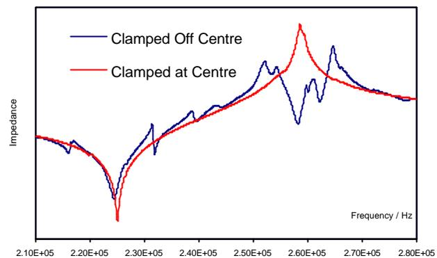
Figure 2: Effects of clamping offset on resonance frequency and spurious peaks.
