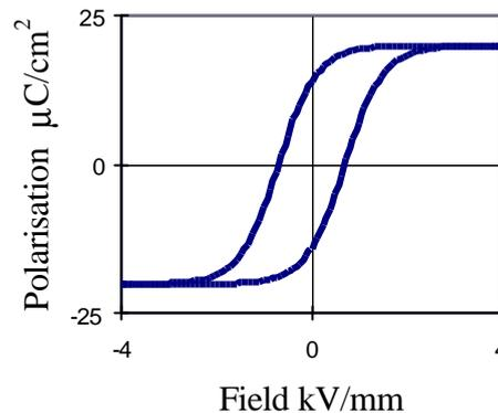
Figure 1b): Non-linear ferroelectric response
