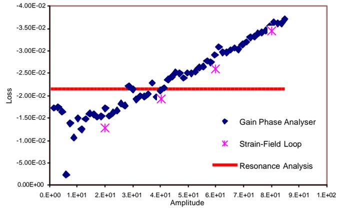
Figure 3: Piezoelectric loss with electric field measured using various techniques.
