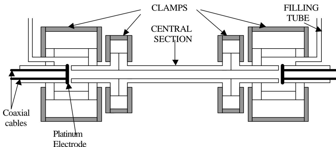
**Figure 1,** Conductivity cell
