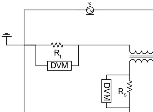
**Figure 4** – Using a current transformer for high current
