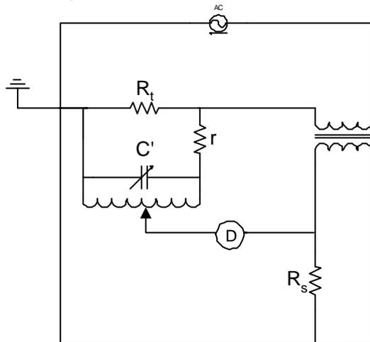
**Figure 2** – Using a resistor to reduce the required capacitance.
