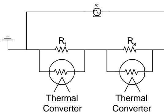
The result of the measurement is the ac/dc difference of the combination of the thermal converter, the shunt and the circuit joining the two components. The effect of the circuit can be assessed by changing the configuration and is usually only a few ppm. The ac/dc difference of the thermal converter is known and is usually small, less than  $5$  ppm.
