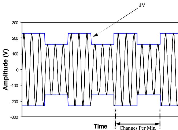
The Flickermeter output depends on the depth of modulation and rate of change of the mains type signal applied to its input. In order to calibrate the Flickermeter it is necessary to characterize such a signal and compare the theoretical response of an ideal Flickermeter to the response of the device being calibrated.
