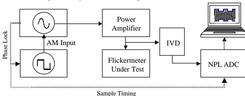
*Figure 3, System for the Calibration of Flickermeters*
