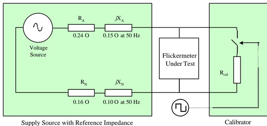
Figure 4, Calibration of a Flicker Test System Using a Calibrator
