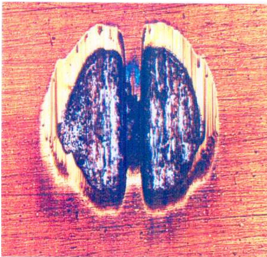
Figure 13 Cleaned wear scar from dry ball cratering sliding wear tests on TiN coated steel sample showing ridging.
