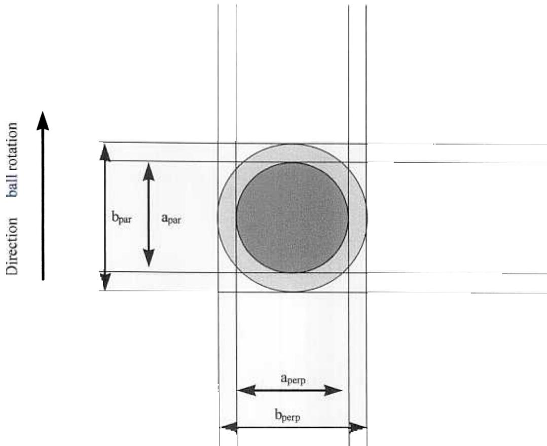
Figure 2 Measurements on wear scar
