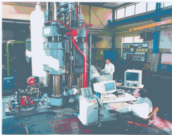
Figure 3. The Big Friction Rig at NPL, interfaced to the 7MN press, used for measurement of friction coefficients under forging conditions.
