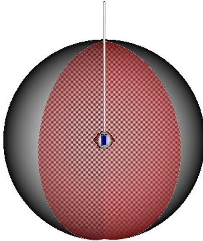
Figure 1: 3D plot of the MCNP geometry of the manganese bath with section removed
