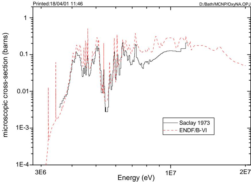
Figure 3: Plot of ENDF/B-VI  $O(n, \alpha)$  cross sections, used by MCNP-4B, and Saclay data, used by the code BATHMCARLO
