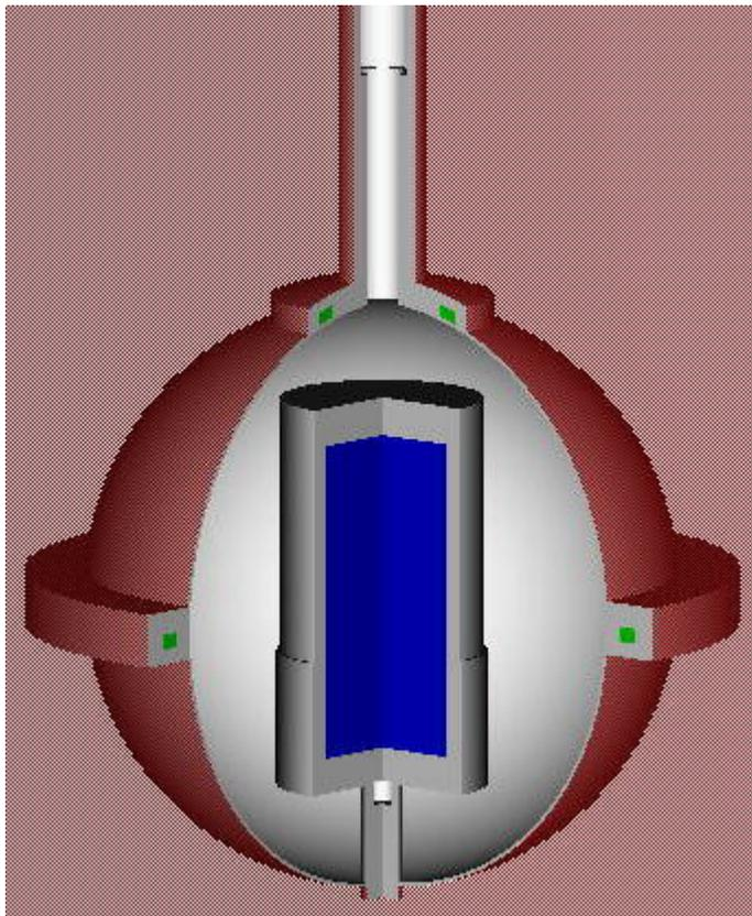
Figure 2: Enlargement of the source cavity containing an X14 capsule
