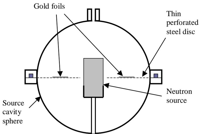
Figure 4: Positions of gold foils inside source cavity (not to scale)
