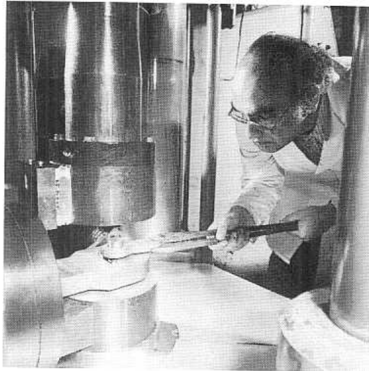
Figure 6. Hot billet being transferred from a furnace to the grabber arm on the Big Friction Rig.
