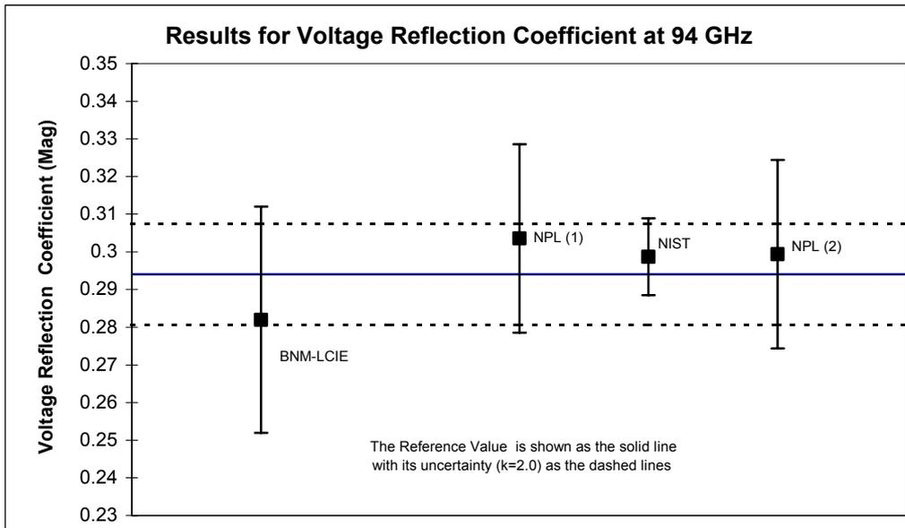
**Figure 2b:** The voltage reflection coefficient magnitude at 94 GHz and its associated expanded uncertainty ( $k = 2.0$ ) given by each of the participating laboratories together with the reference value and its associated uncertainty ( $k = 2.0$ ).
