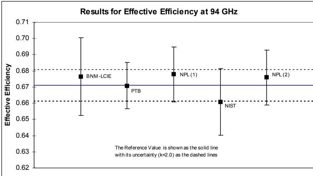
**Figure 2a:** The effective efficiency at 94 GHz and its associated expanded uncertainty ( $k = 2.0$ ) given by each of the participating laboratories together with the reference value and its associated uncertainty ( $k = 2.0$ ).
