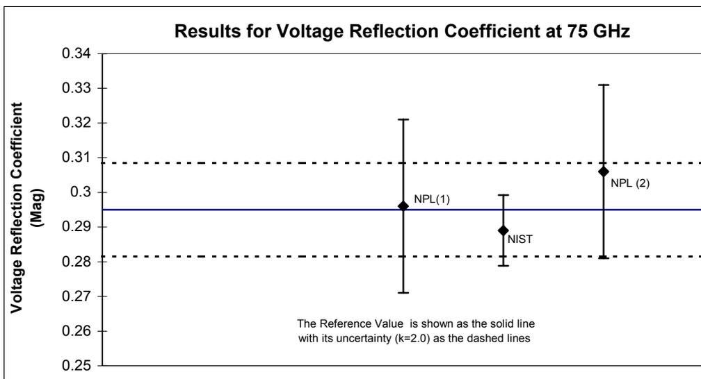
**Figure 1b:** The voltage reflection coefficient magnitude 75 GHz and its associated expanded uncertainty ( $k=2.0$ ) given by each of the participating laboratories together with the reference value and its associated uncertainty ( $k=2.0$ ).
