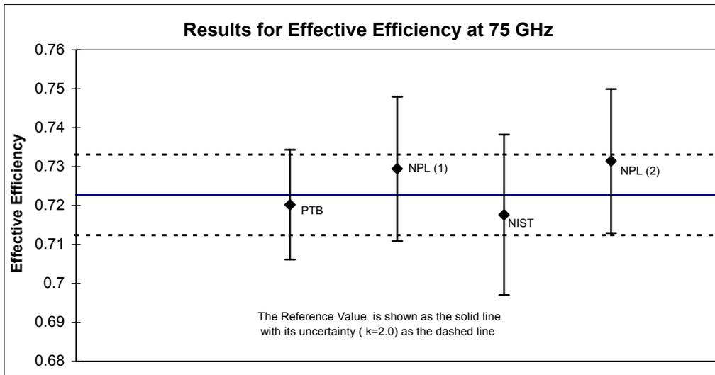
**Figure 1a:** The effective efficiency at 75 GHz and its associated expanded uncertainty ( $k=2.0$ ) given by each of the participating laboratories together with the reference value and its associated uncertainty ( $k=2.0$ ).
