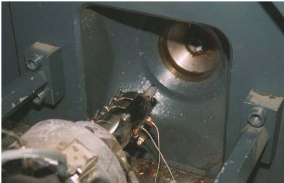
Figure 4. Schematic diagram and photograph of an instrumented nozzle on an injection moulding machine.
