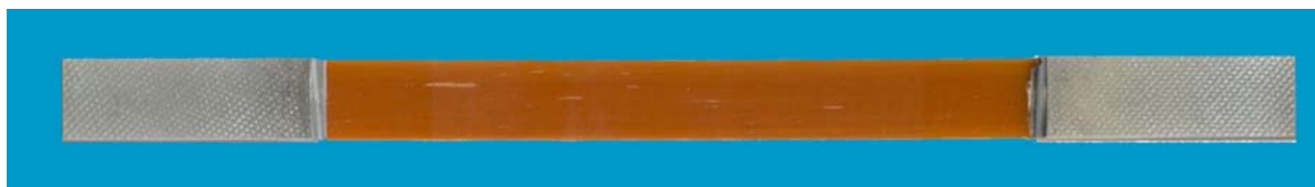
Figure 9: Fibre debonding and matrix cracking in unidirectional E-glass/913 (narrow, whitened areas along gauge-length indicate damage).
