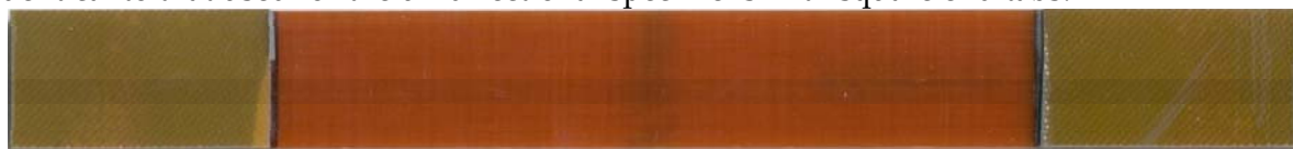
Figure 3: Straight-sided cross-ply specimen with bonded end tabs.
