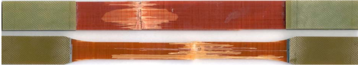
Figure 17: Typical failures for the straight-sided and dumbbell specimen types.
