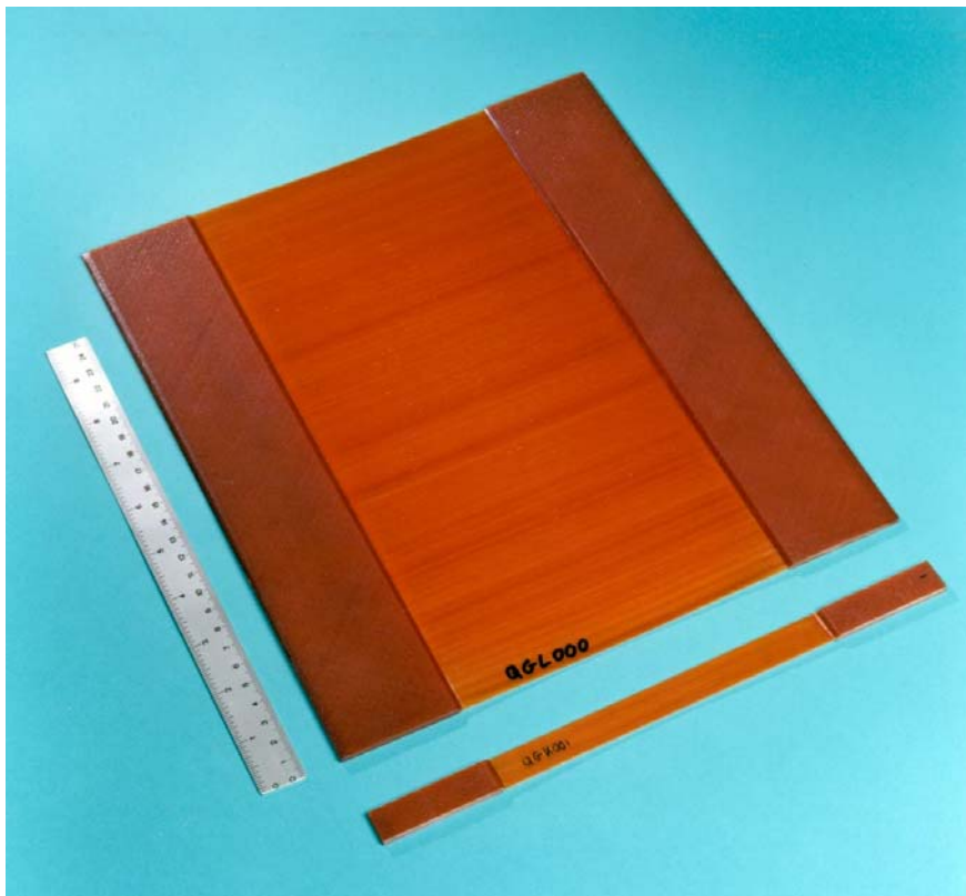
Figure 2: Unidirectional E-glass/913 laminate with in-built end tabs.
