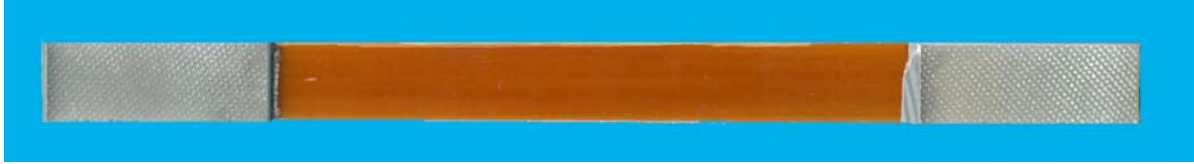
Figure 10: Edge damage in unidirectional E-glass/913.
