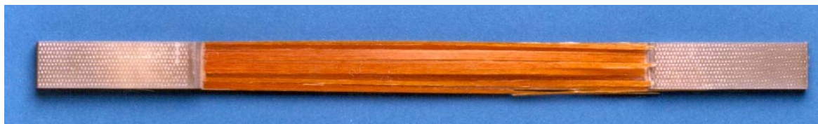
Figure 8: Typical tension-tension fatigue failure for unidirectional E-glass/913 laminate.
