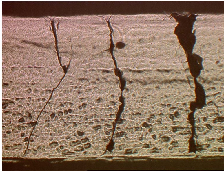
Figure 21: Magnified image of transverse cracks along an edge of a cross-ply laminate.
