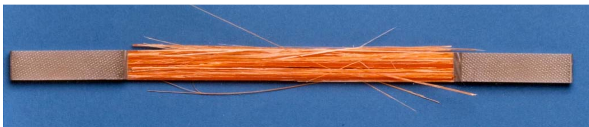
Figure 7: Typical tensile failure for unidirectional E-glass/913 laminate.
