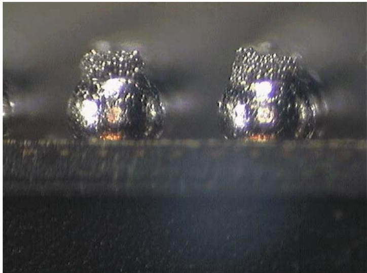
**Figure 5. Re-balling of BGAs following a print stage, side view**
