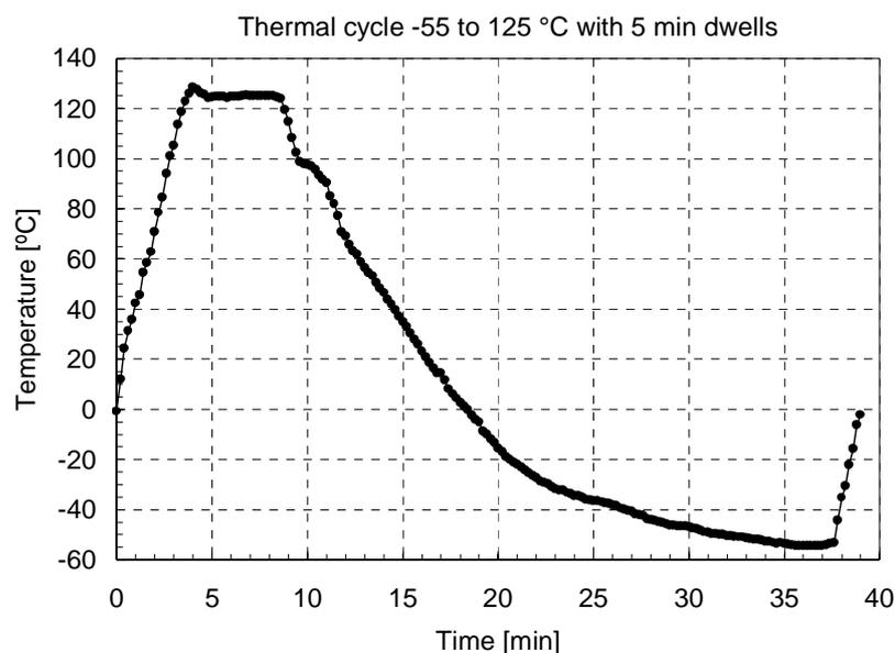
**Figure 3. Temperature cycle load used**
