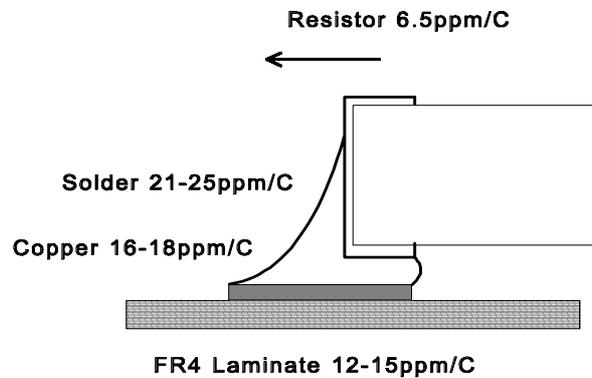
**Figure 1. TCE (X-axis) mismatches in SM assemblies**
