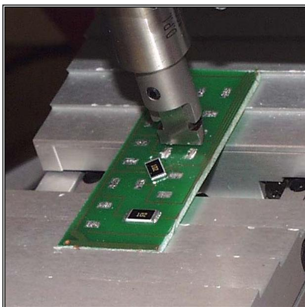
**Figure 5. Typical joint break after failure**
