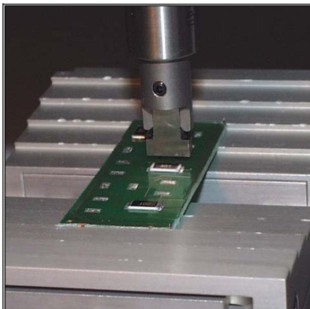
**Figure 4. Shear test jig and push-off tool.**
