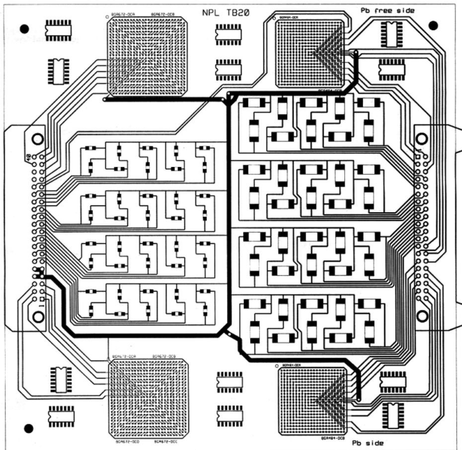
Figure 2. Example of test pcb layout, size 152 x 152 x 1.6 mm
