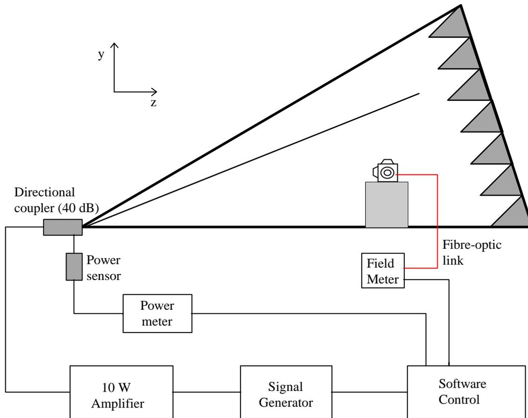
**Figure 5 : Experimental set-up of the isotropic probe in the GTEM**
