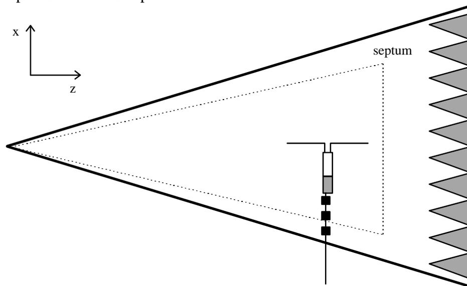
**Figure 4 : Schematic diagram showing position of dipole and cables for cross-polar measurements**
