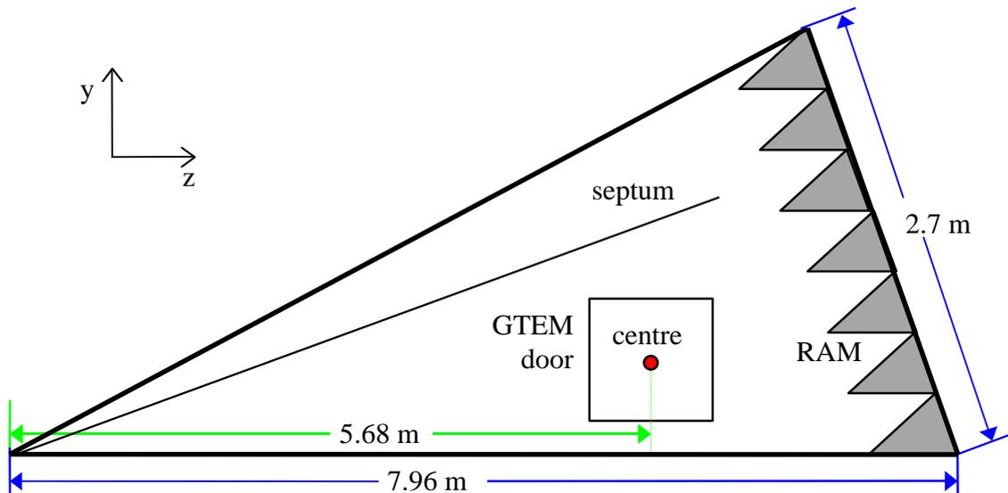
Figure 1 : Dimensions of GTEM, side cutaway through centre
