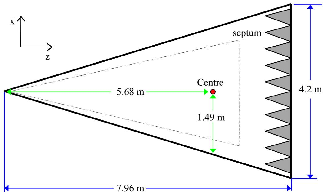
Figure 2 : Dimensions of GTEM, plan view
