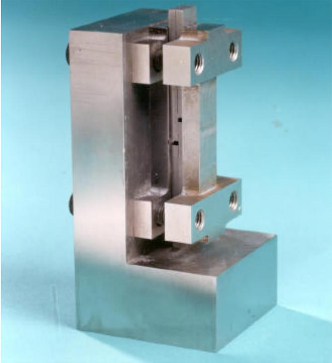
Figure 4 Support fixture with specimen.
