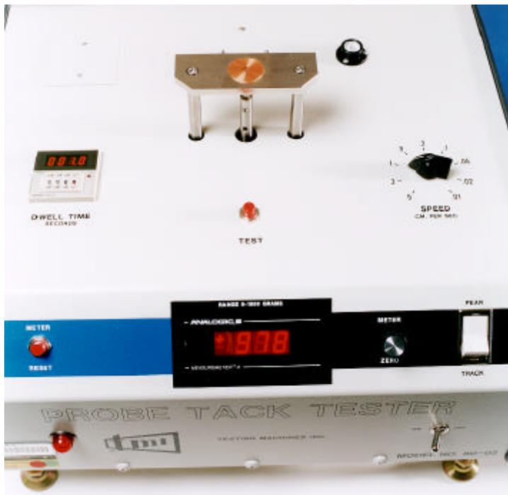
**Figure 2: Probe tack tester**
