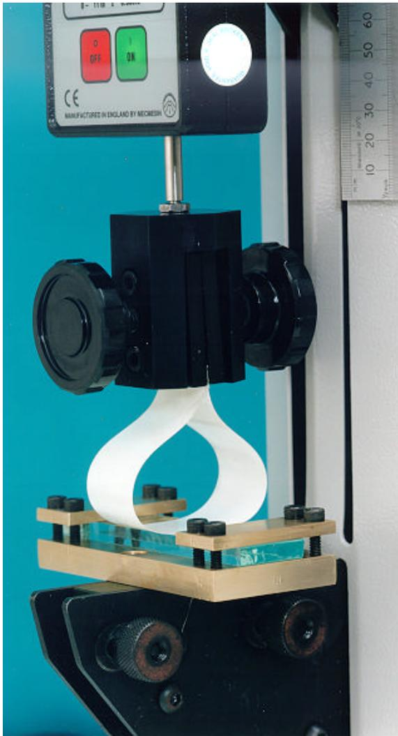
**Figure 1: Loop tack test**
