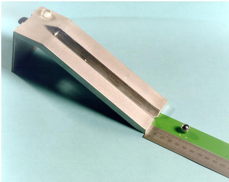
**Figure 3: Rolling ball tack test**
