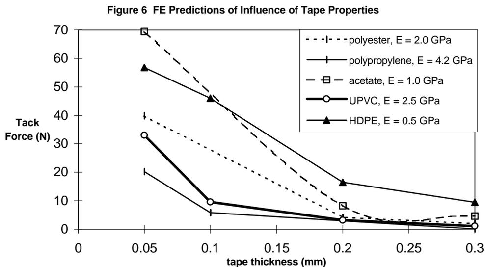
Figure 6 summarises the initial predictions made. The main trend is that the measured force will decrease as the stiffness of the tape increases. This does not take into account the higher contact pressures produced by the stiffer tapes that would tend to increase the measured tack.
