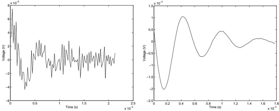
**Figure 7:** Incorporating *a priori* information about the drive voltage  $f_0$  by filtering. A filter is applied to the data in the time-window  $[t_0, t_2]$  comprising  $m = 112$  points with (a)  $l = 1$  (left), and (b)  $l = 10$  (right).
