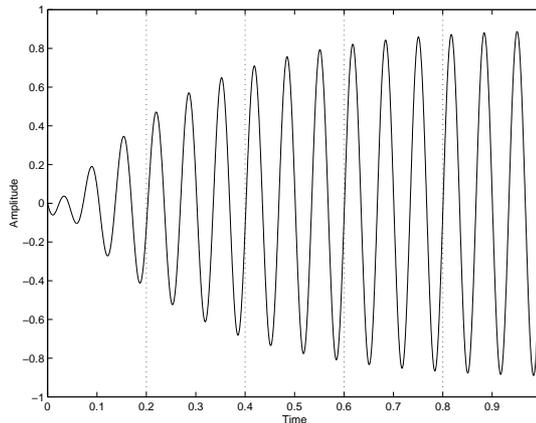
**Figure 3:** An example of a normalised waveform for a moderately high- $Q$  transducer driven at its resonance frequency. Note that steady-state is not reached within the available time window.
