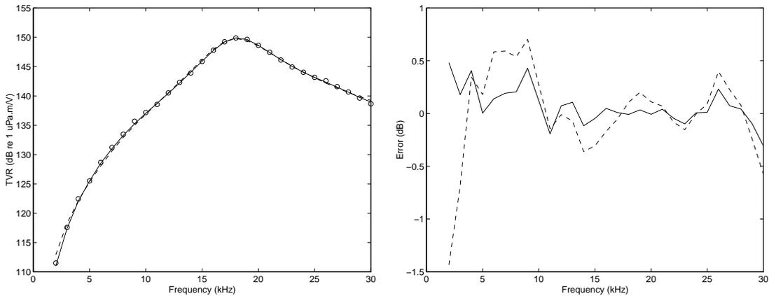
**Figure 13:** On the left, transmitting voltage responses from (i) free field measurements (small circles), (ii) measurements from a time-window comprising  $m = 112$  points (solid line), and (iii) measurements from a time-window comprising  $m = 56$  points (dashed line). On the right, the differences between (i) and (ii) (solid line), and between (i) and (iii) (dashed line).
