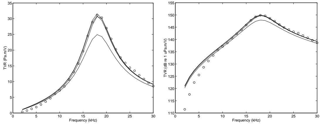
**Figure 14:** Transmission voltage responses obtained from estimates of the resonant behaviour of the device. Each curve is derived from the analysis of data corresponding to a single drive frequency. The data analysed was contained within the time-window  $[t_0, t_2]$  comprising  $m = 112$  points.
