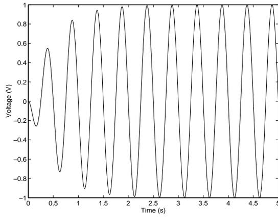
**Figure 10:** Simulated data representing the response of a device when driven at its resonance frequency.
