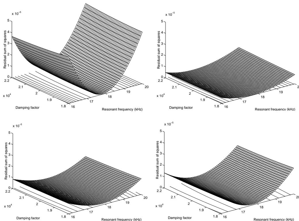
**Figure 4:** Residual sum of squares as a function of the resonance frequency and damping factor for the ITC1001 transducer and the cases (a)  $f_0 = 18$  kHz,  $m = 112$  (top-left), (b)  $f_0 = 18$  kHz,  $m = 56$  (top-right), (c)  $f_0 = 11$  kHz,  $m = 112$  (bottom-left), and (d)  $f_0 = 25$  kHz,  $m = 112$  (bottom-right). The functions are displayed as 3D surfaces above corresponding contour plots.
