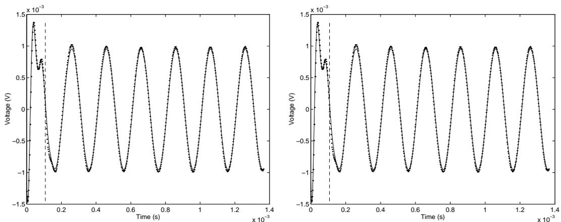
**Figure 9:** Estimates of the voltage output obtained by fitting the data in the time-window  $[t_0, t_1]$  comprising  $m = 56$  points using non-linear estimation and (a) the weighted least-squares Prony method (left), and (b) the least-squares Prony-SVD method (right), to provide starting estimates.
