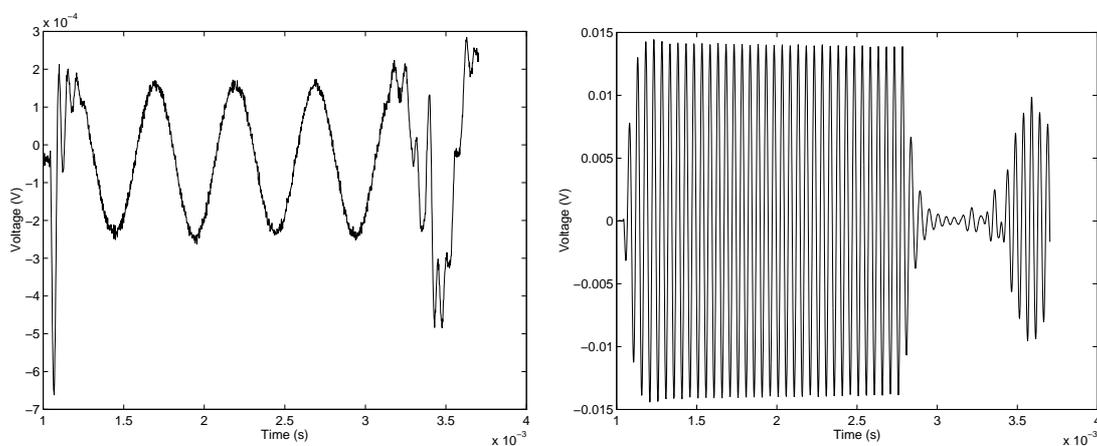
**Figure 2:** Measured data for the ITC1001 transducer corresponding to a 2 kHz drive voltage (left), and a 20 kHz drive voltage (right).
