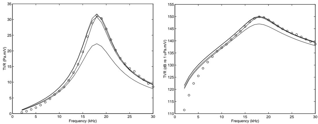
**Figure 15:** Transmission voltage responses obtained from estimates of the resonant behaviour of the device. Each curve is derived from the analysis of data corresponding to a single drive frequency. The data analysed was contained within the time-window  $[t_0, t_1]$  comprising  $m = 56$  points.
