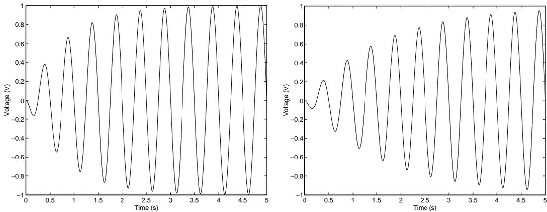
**Figure 12:** Simulated data representing the response of devices with different  $Q$ -factors and driven at their resonance frequency.
