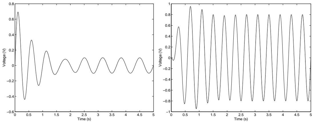
**Figure 11:** Simulated data representing the response of a device at frequencies below (on the left) and above (on the right) its resonance frequency.
