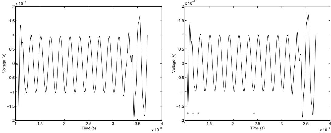
**Figure 6:** Data for the ITC1001 transducer corresponding to a 5 kHz drive voltage: (a) acquired data (left), and (b) after removal of background dc level (right).
